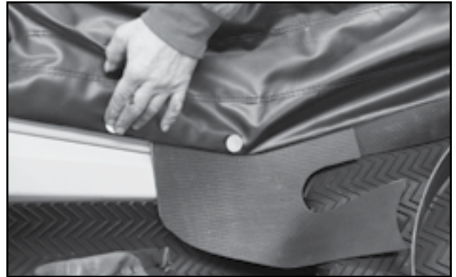
Fig 90 - Corner flashing
