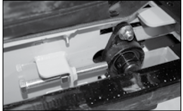
Fig 73 - Adjustment Bolt on Open Transition Hopper
