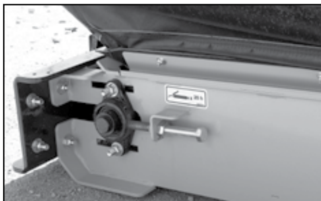
Fig 52 - Tail roller bearing
