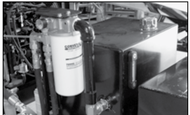
Fig 82 - Hydraulic Oil Filter
