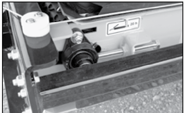
Fig 55 - Hopper Roller Bearings
