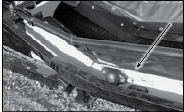
Fig 56 - Transition Roller Bearings
