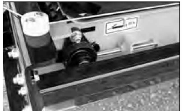
Fig 53 - Hopper Roller Bearings
