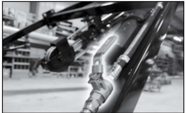
Fig 38 - Hydraulic Valve to Lift Cylinder
