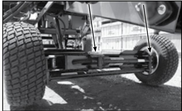
Fig 62 - Steering wheel axle bushings
