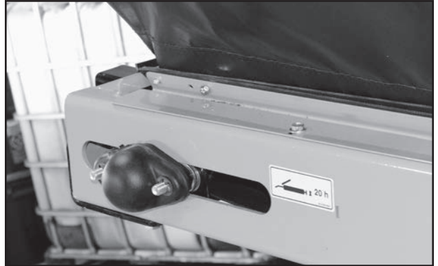
Fig 52 - Hopper Bearings
