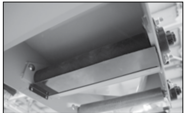
Fig 79 - Containment plate in place
