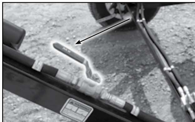
Fig 16 - Hydraulic valve to the lift cylinder
