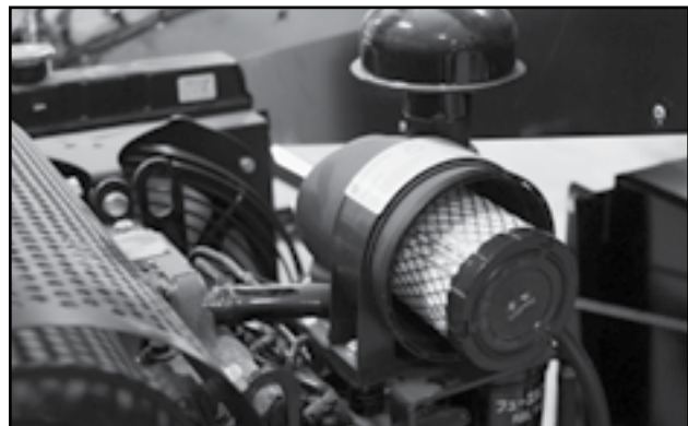
Fig 81 - Donaldson Air Filter, Cover Removed
