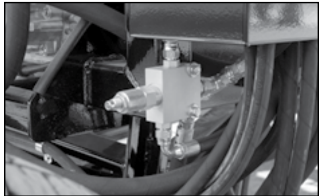
Fig 51 - Cushion Block below valve table
