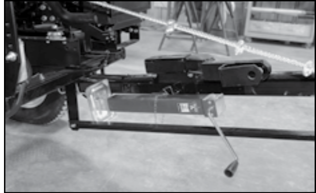
Fig 46 - Drawbar and jack storage plate
