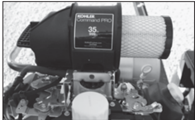
Fig 81 - Kohler Air Filter, Cover Removed
