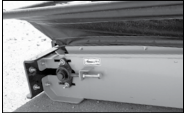
Fig 57 - Tail roller bearing
