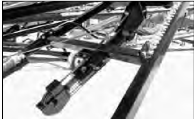
Fig 66 - Conveyor Lift Cylinder
