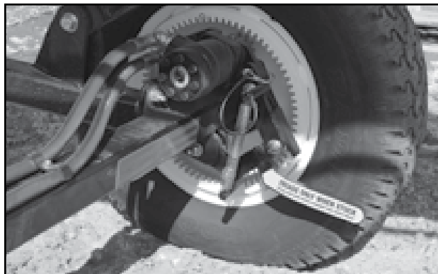
Fig 25 - Disengaged Drive Wheel
