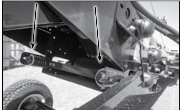
Fig 71 - Spring tension bolt
