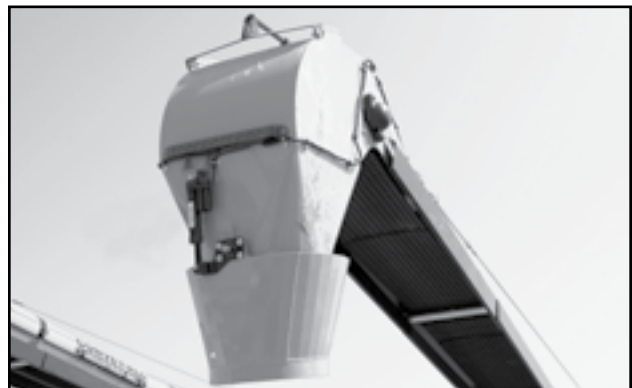
Fig 27 - Quad-swivel discharge spout and transport lights
