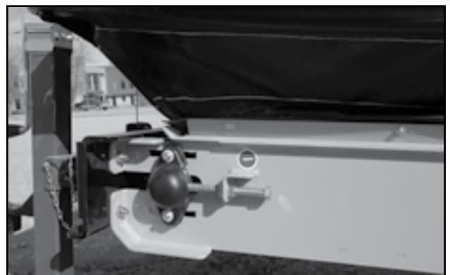
Fig 73 - Adjustment bolt at tail roller
