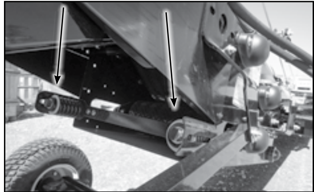
Fig 71 - Spring tension bolt
