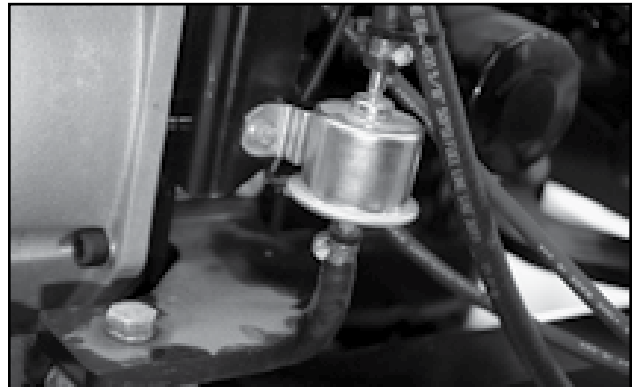
Fig 81 - In-Line Fuel Filter, Diesel Engine
