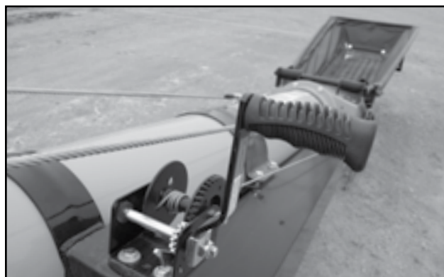
Fig 22 - Hopper winch
