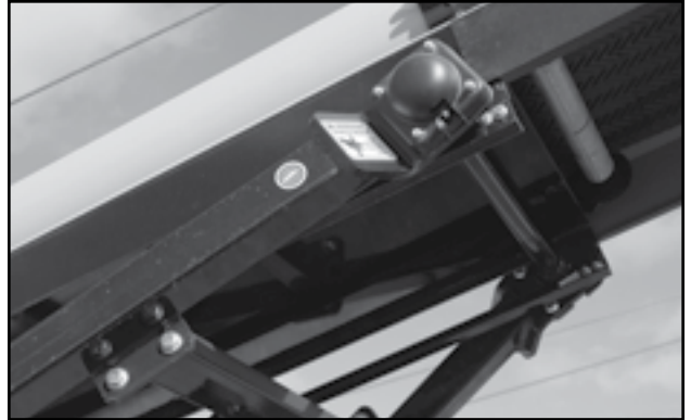
Fig 67 - Upper lift bearings
