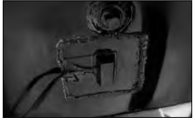
Fig 26 - Oil Tank Heater, bottom of Reservoir
