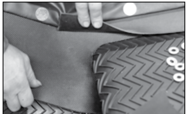
Fig 92 - Corner flashing tight around roller
