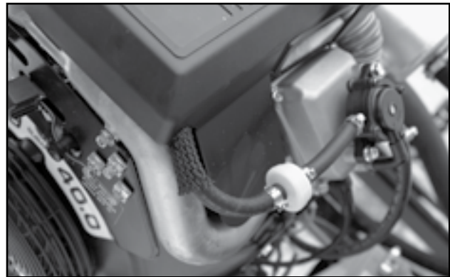
Fig 62 - In-line Fuel Filter
