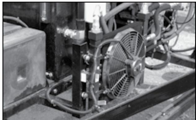
Fig 13 - Oil cooler
