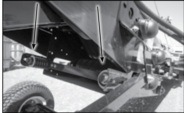
Fig 55 - Tension bolts, below drive box
