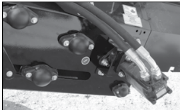
Fig 58 - Conveyor belt hydraulic drive motor
