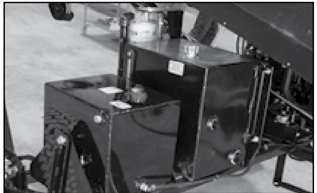
Fig 54 - Fuel Tank and Hydraulic Oil Reservoir
