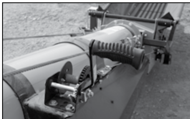
Fig 22 - Hopper winch
