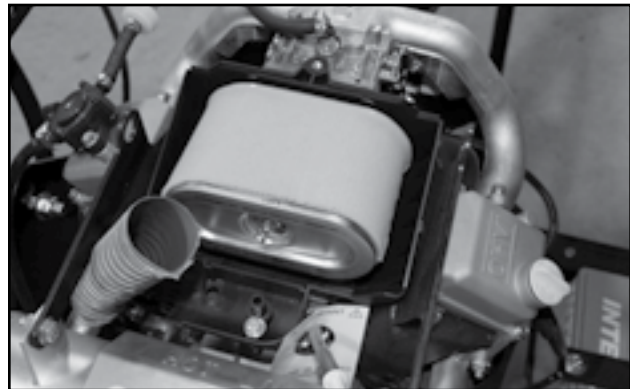
Fig 80 - Foam Air Filter, Cover Removed
