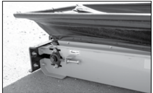
Fig 73 - Adjustment bolt at tail roller
