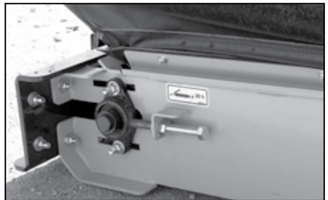
Fig 54 - Tail roller bearing
