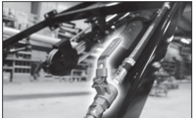
Fig 39 - Hydraulic Valve to Lift Cylinder
