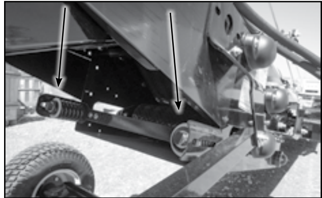
Fig 69 - Spring tension bolt
