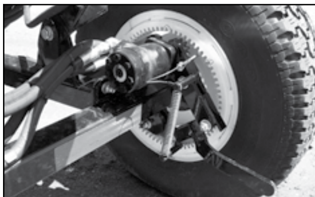
Fig 44 - Disengage drive wheels
