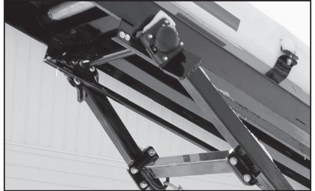
Fig 68 - Upper Lift Bearings
