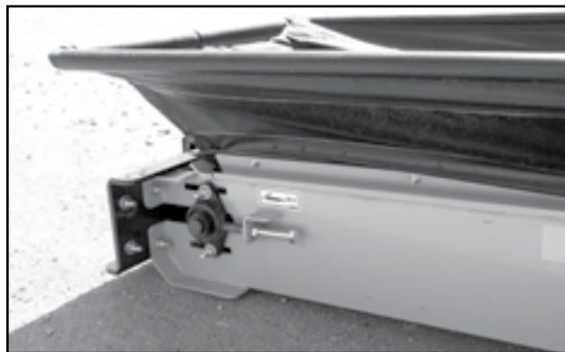
Fig 71 - Adjustment bolt at tail roller
