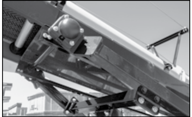
Fig 65 - Steering wheel lift cylinder
