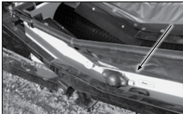
Fig 54 - Transition Roller Bearings
