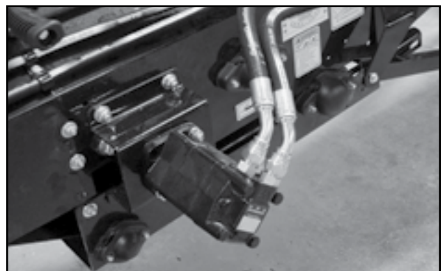
Fig 60 - Conveyor Belt Drive Motor
