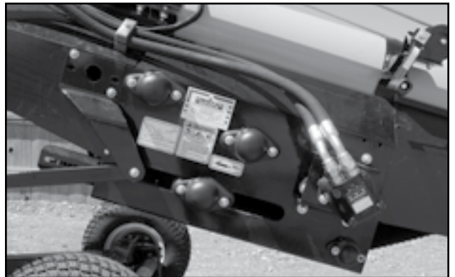
Fig 59 - Drive box roller bearings
