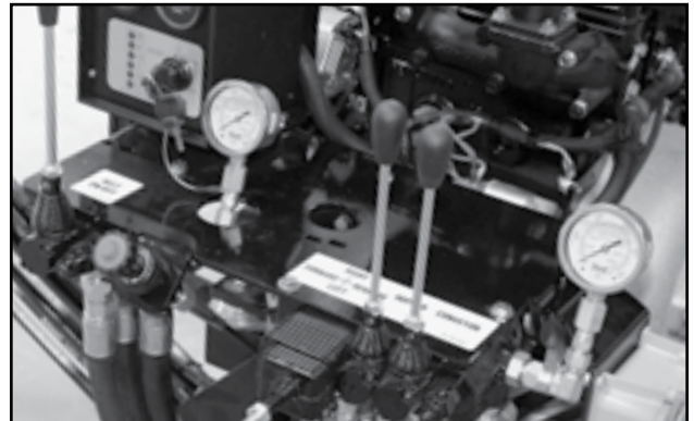
Fig 12 - Hydraulic Pressure Gauges
