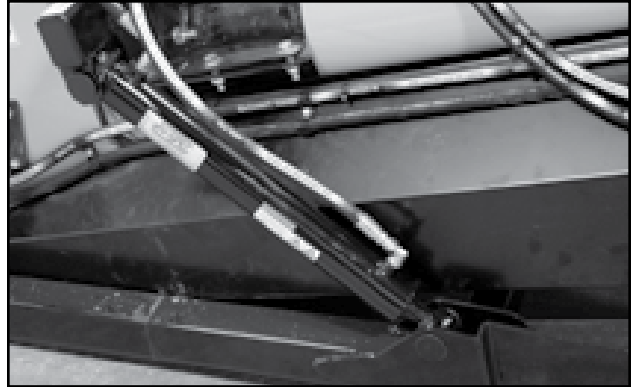
Fig 67 - Steering Wheel Lift Cylinder
