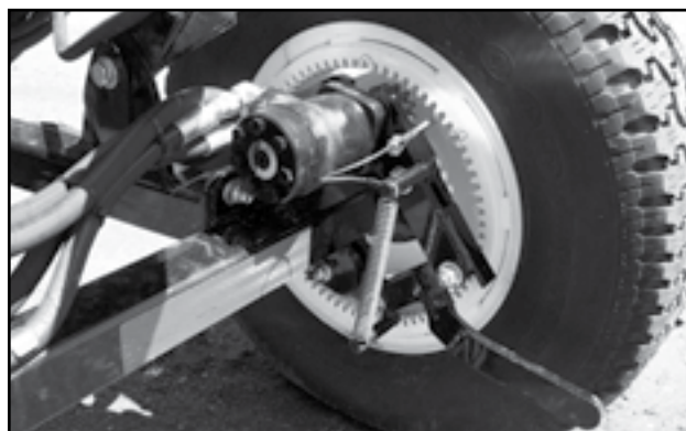
Fig 44 - Disengage drive wheels
