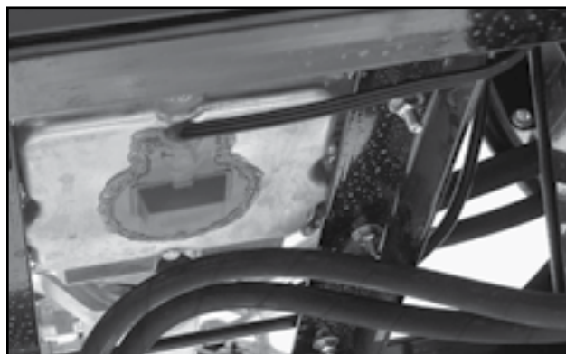
Fig 9 - 125 watt heater for engine
