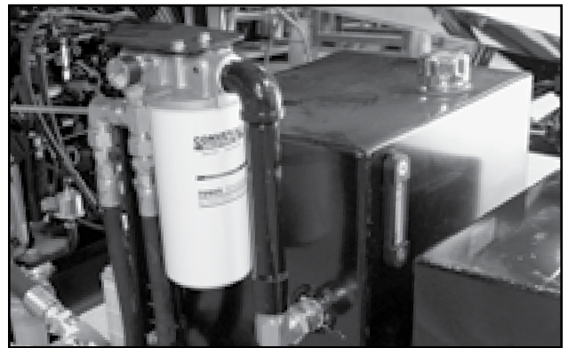
Fig 84 - Hydraulic Oil Filter
