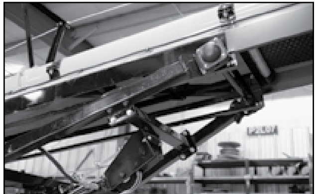
Fig 69 - Upper Lift Bearings
