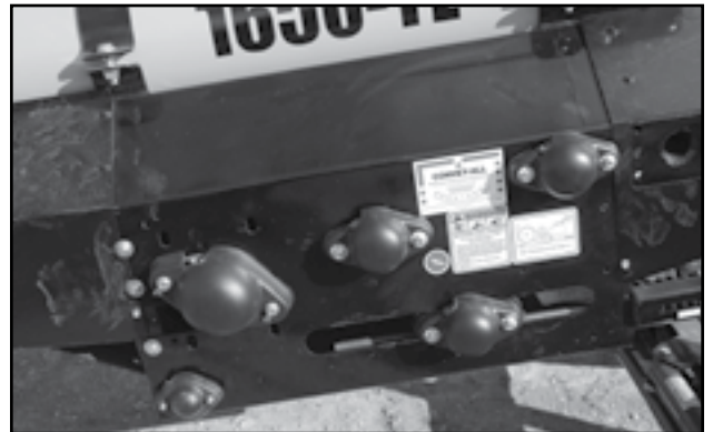
Fig 61 - Drive box roller bearings
