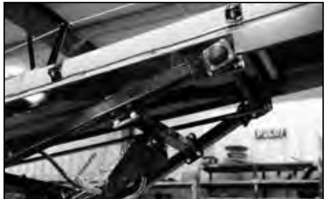
Fig 67 - Upper Lift Bearings
