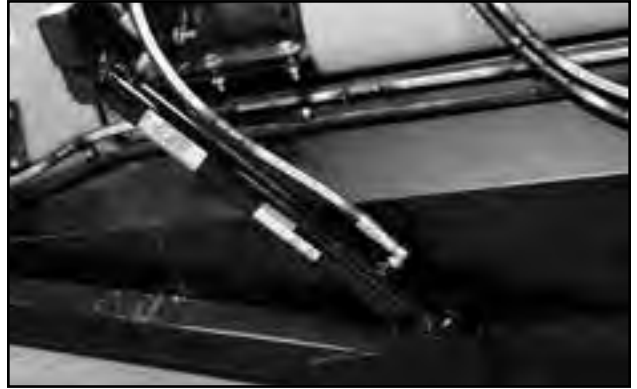
Fig 65 - Steering Wheel Lift Cylinder
