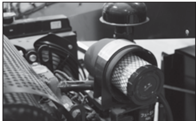
Fig 82 - Donaldson Air Filter, Cover Removed
