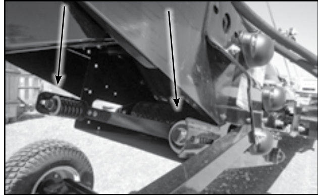
Fig 53 - Tension bolts, below drive box
