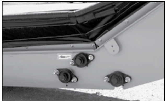
Fig 58 - Transition roller bearings
