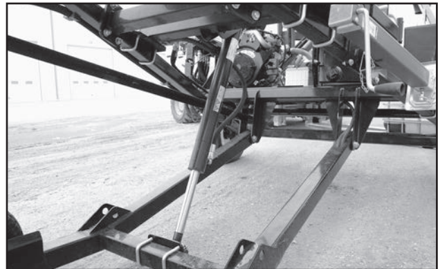
Fig 66 - Steering Wheel Lift Cylinder
