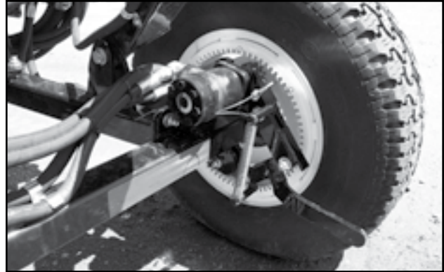
Fig 17 - Disengaged drive wheel
