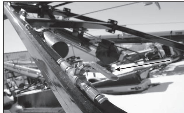
Fig 13 - Hydraulic Valve to the Lift Cylinder
