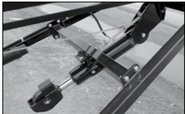
Fig 66 - Conveyor lift cylinder
