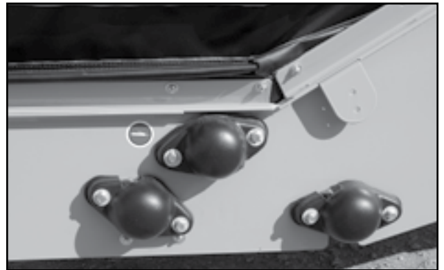
Fig 60 - Transition roller bearings
