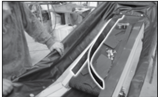
Fig 88 - Layer side flashing pieces
