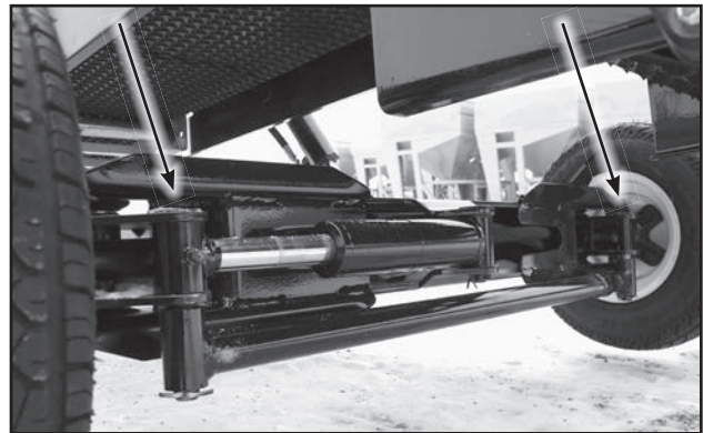
Fig 65 - Steering Wheel Axle Bushing
