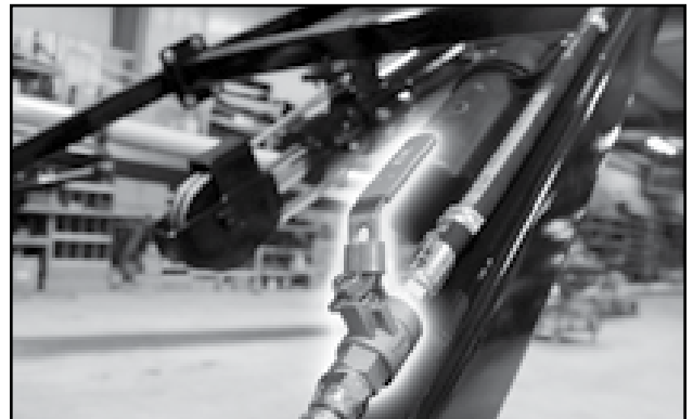
Fig 40 - Hydraulic Valve to Lift Cylinder
