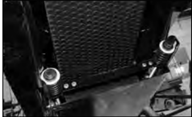
Fig 73 - Spring Tension Bolts
