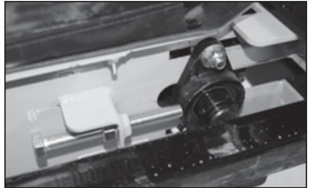
Fig 72 - Adjustment Bolt on Open Transition Hopper
