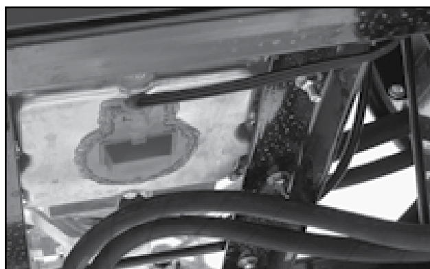
Fig 9 - 125 Watt Heater for Engine
