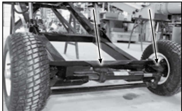
Fig 64 - Steering Wheel Axle Bushings
