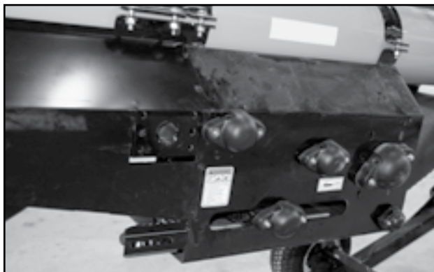
Fig 55 - Drive Box Roller Bearings
