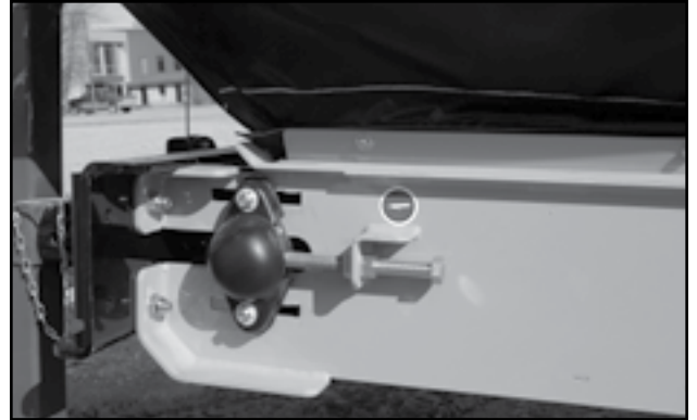
Fig 59 - Tail roller bearing
