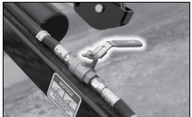
Fig 40 - Hydraulic valve to lift cylinder
