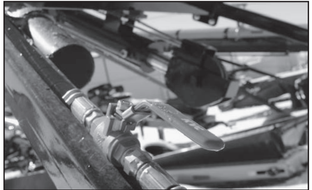
Fig 38 - Hydraulic Valve to Lift Cylinder
