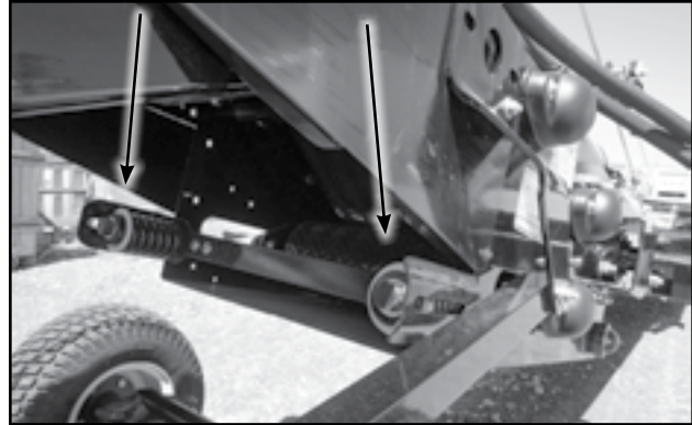
Fig 55 - Tension bolts, below drive box
