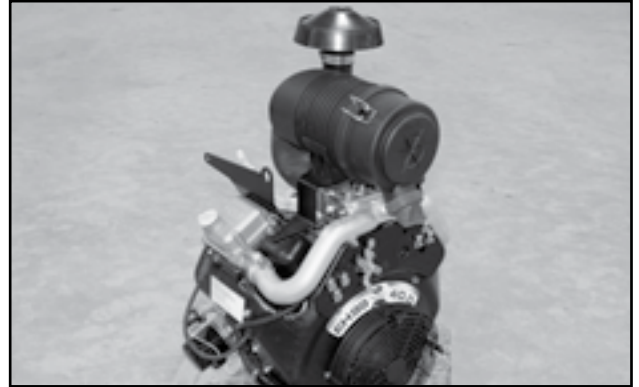
Fig 4 - Subaru Gas Engine with Donaldson Air Filter
