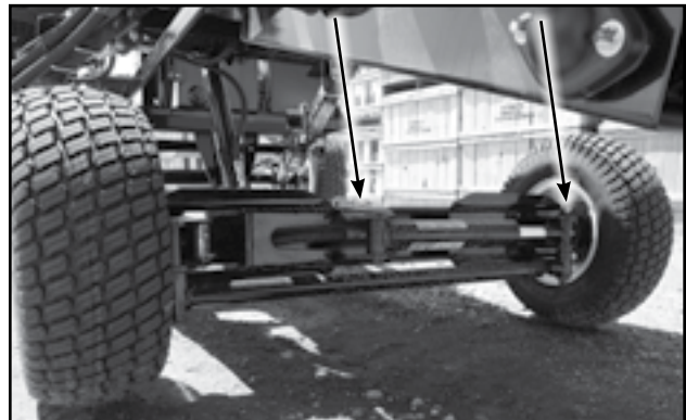
Fig 64 - Steering wheel axle bushings
