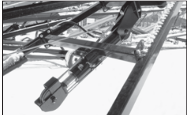
Fig 67 - Conveyor Lift Cylinder
