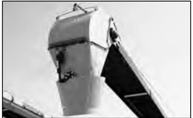
Fig 19 - Quad-Swivel Discharge Spout
