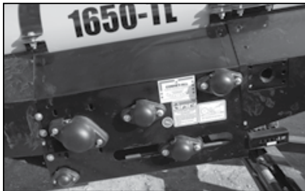
Fig 54 - Drive box roller bearings
