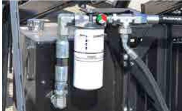
Fig 96 - Hydraulic oil filter
