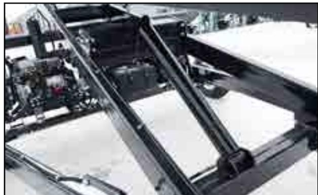
Fig 75 - Conveyor tube lift cylinder
