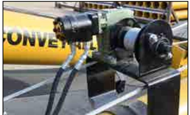
Fig 35 - Hydraulic winch
