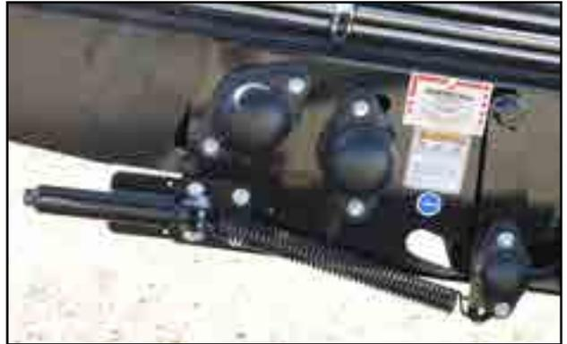
Fig 69 - Positive pinch drive tension bolts
