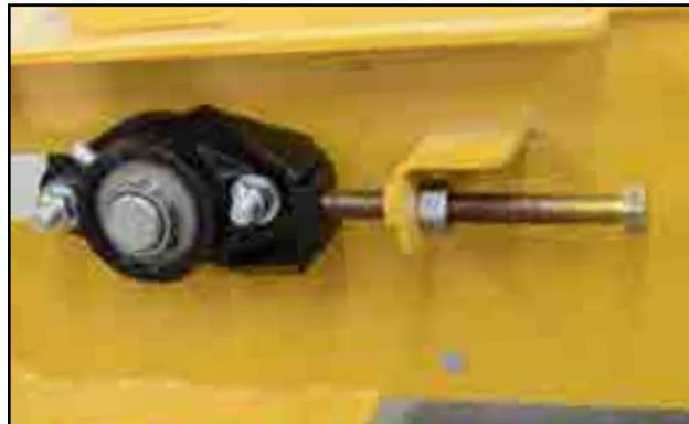
Fig 87 - Swing-out hopper idler roller and adjustment bolt
