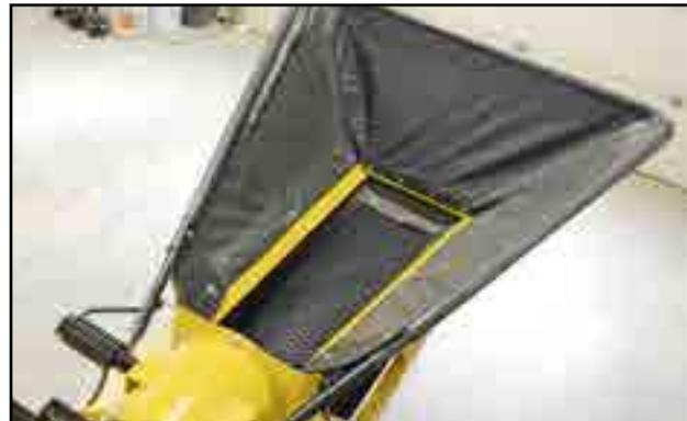
Fig 66 - Collapsible main conveyor hopper
