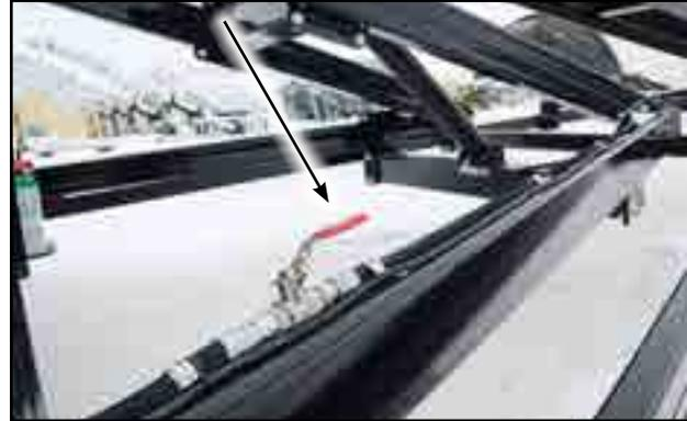
Fig 15 - Hydraulic ball valve to the lift cylinder
