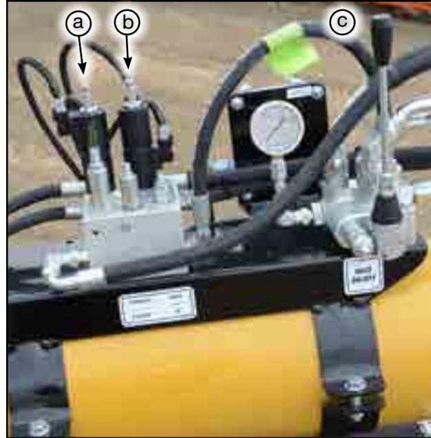
Fig 44 - Remote control valve table
