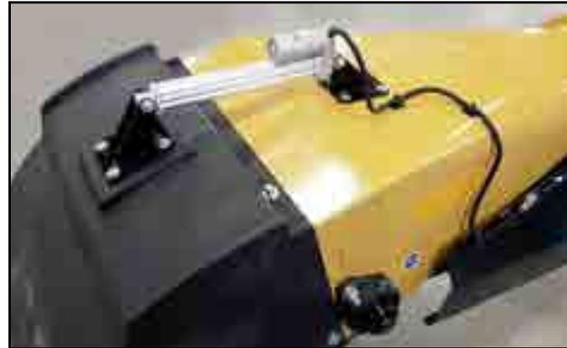
Fig 24 - Electric actuator
