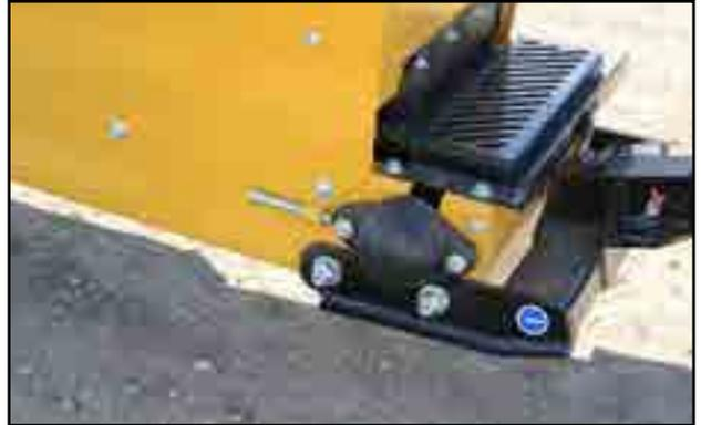
Fig 68 - Adjustment bolts on side of hopper
