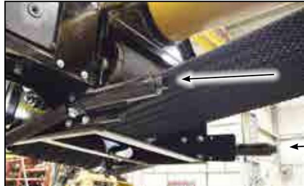
Fig 80 - Tension Bolt
