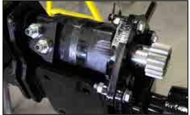
Fig 112 - Pinion gear
