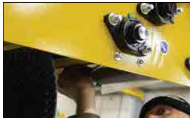
12. Link the ends of the new belt lacing.
