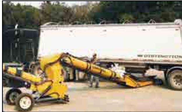
Fig 55 - Trailer unloading into swing-out conveyor
