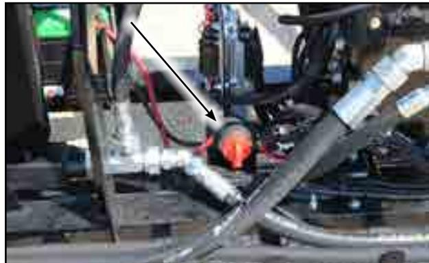
Fig 9 - Power shut-off switch
