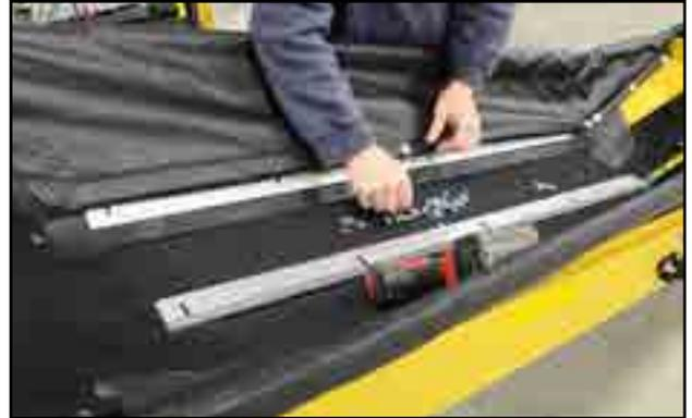
Fig 105 - Stainless steel Hold-Down Strip Plates
