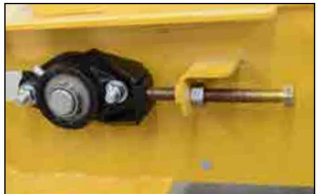
Fig 82 - Swing-out hopper idler roller and adjustment bolt
