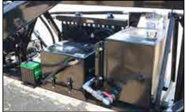
Fig 62 - Hydraulic oil reservoir and fuel tank
