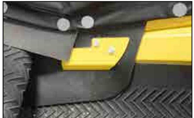
Fig 107 - Fasten flashing clamp
