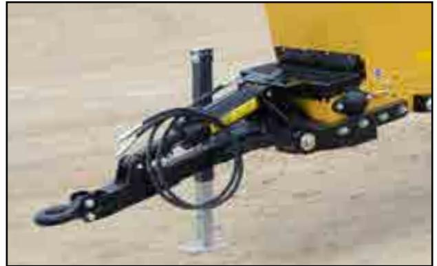
Fig 49 - Hydraulic hitch
