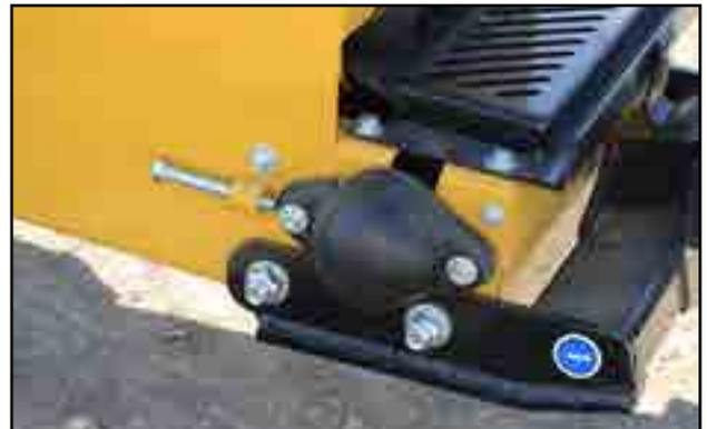
Fig 64 - Hopper roller bearings
