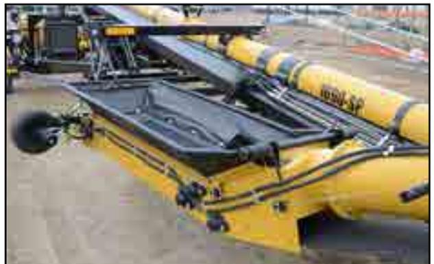
Fig 71 - Swing-out conveyor
