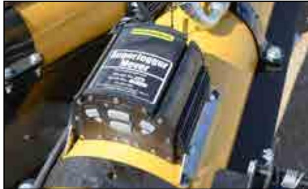
Fig 39 - Auger Jogger receiver box
