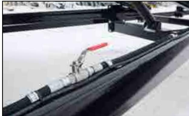
Fig 53 - Hydraulic ball valve to tube lift cylinder
