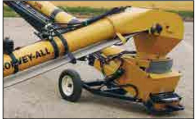
Fig 34 - Discharge of swing-out with manual winch
