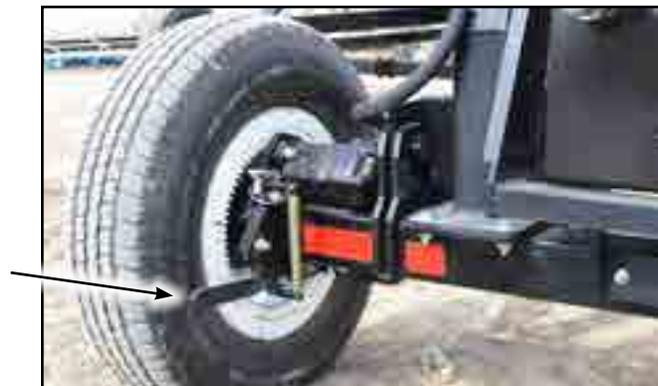
Fig 17 - Drive wheel and engagement lever
