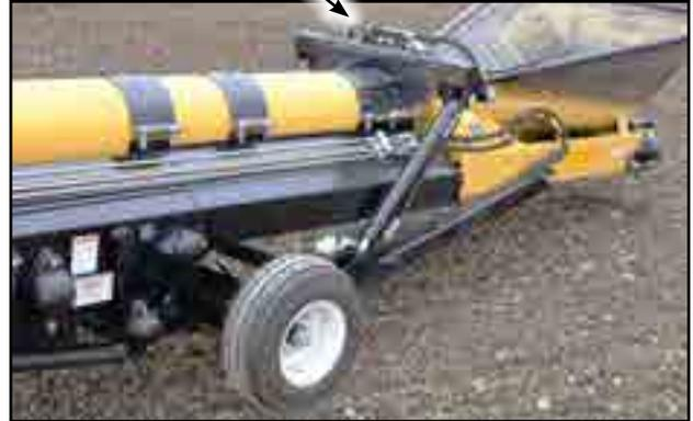
Fig 19 - Steering wheels. Check valve on cylinder mount
