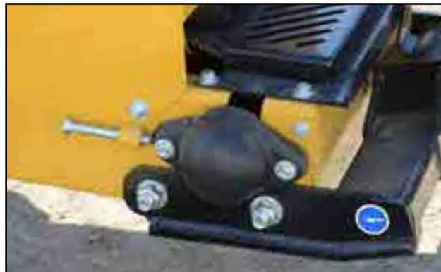
Fig 83 - Adjustment bolt on side of hopper
