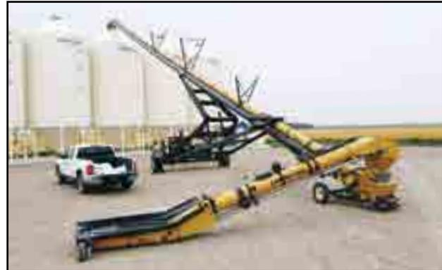
Fig 31 - Swing-out conveyor (optional)
