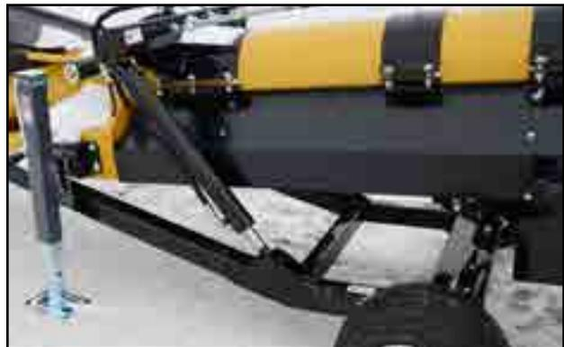
Fig 74 - Steering wheel lift cylinder
