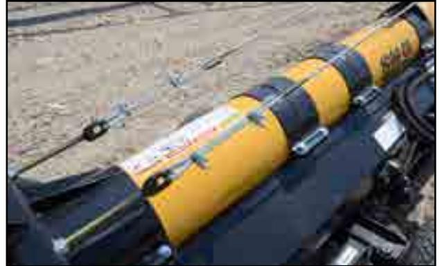
Fig 76 - Eyebolts and cable bridging
