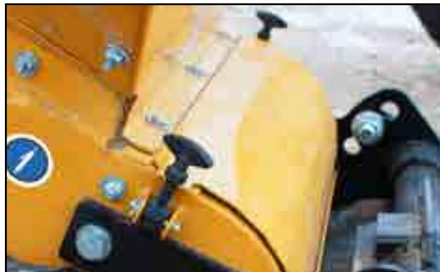
Fig 41 - Hopper end belt, guard in place
