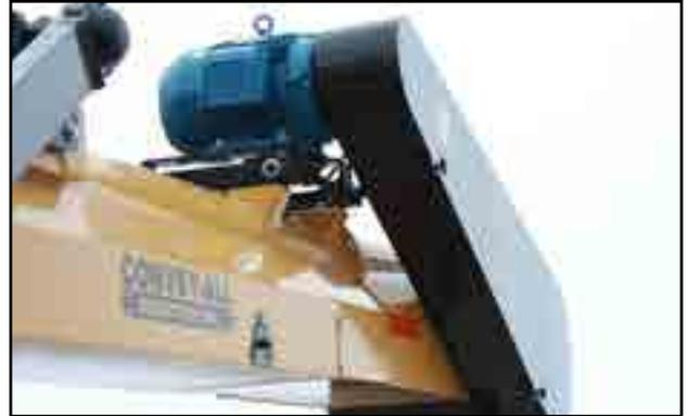
Fig 6 - Electric motor with direct drive
