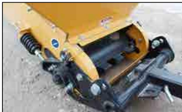
Fig 13 - Adjustable hitch. Belt guard is shown removed
