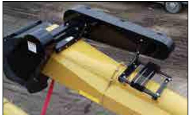
Fig 7 - Speed reducer with counter shaft
