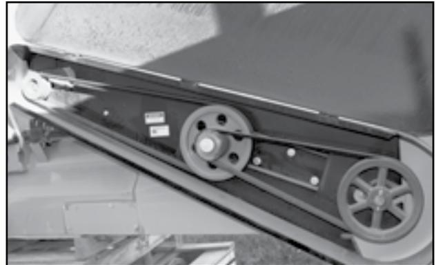
Fig 51 - In-Line Drive with Guard Opened
