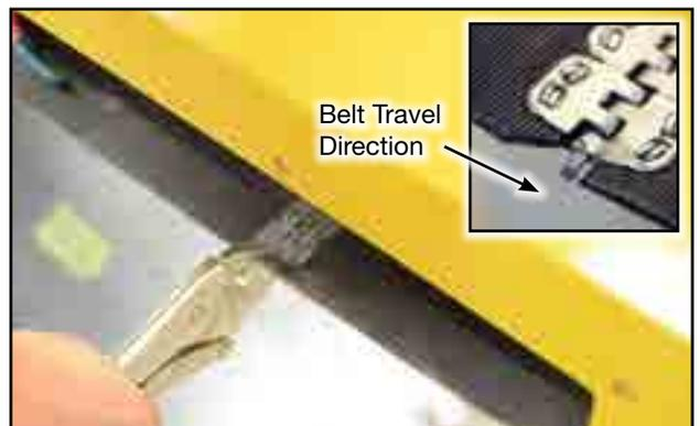
Fig 46 - Crimp lacing and taper belt corner
