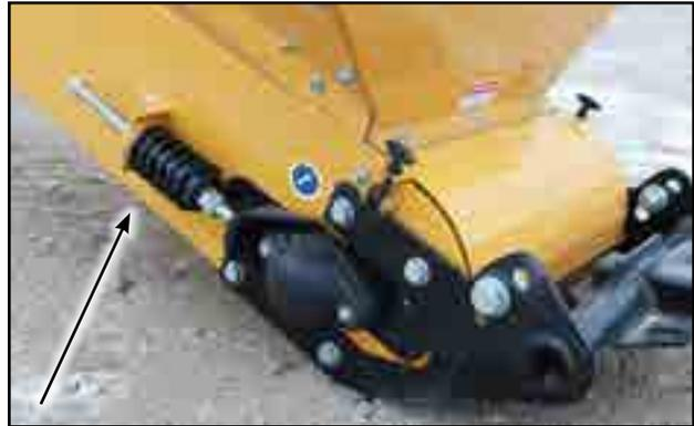
Fig 23 - Tension spring
