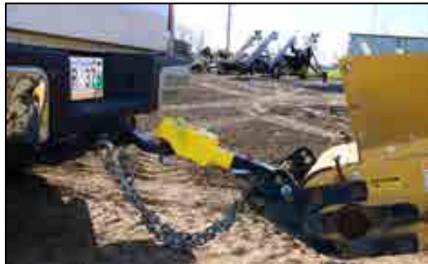
Fig 29 - Ball hitch with safety chains
