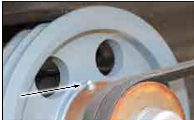
Fig 34 - Grease zerk on pulley
