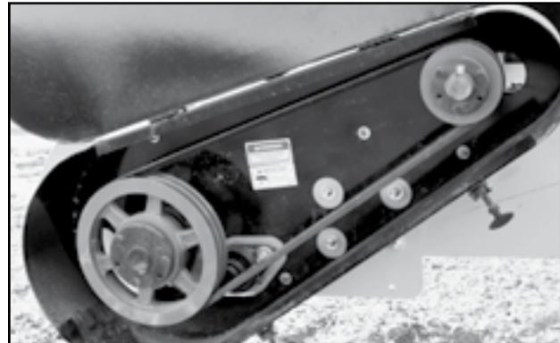
Fig 48 - Speed Reduction Drive with Guard Opened
