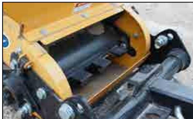
Fig 42 - Hopper end belt, guard removed
