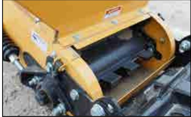
Fig 22 - Hopper end belt guard removed
