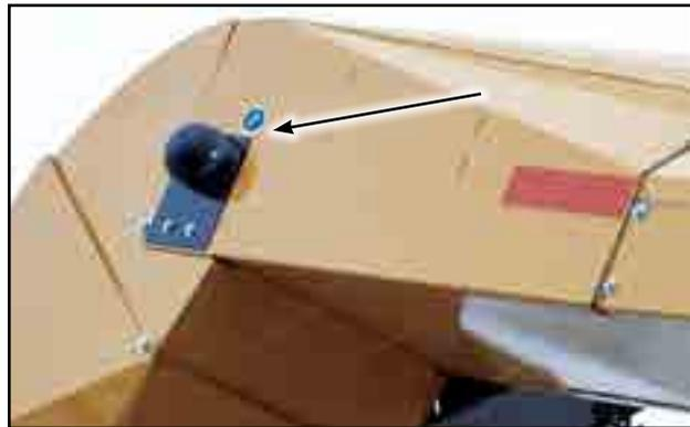
Fig 33 - Discharge roller bearings
