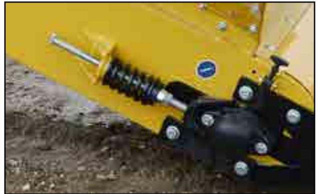
Fig 40 - Adjustment bolt and tension spring
