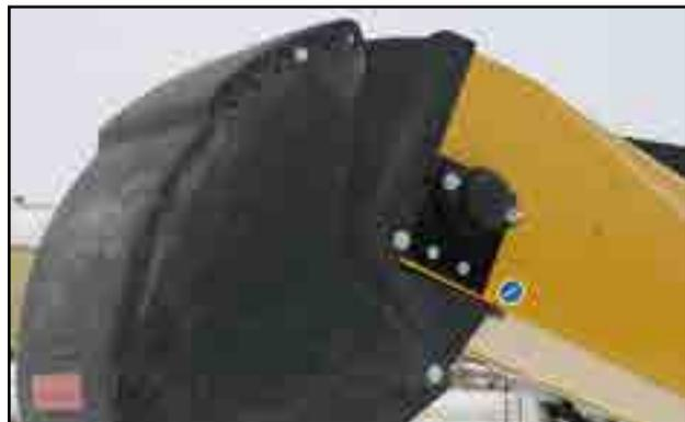
Fig 39 - Discharge bearing
