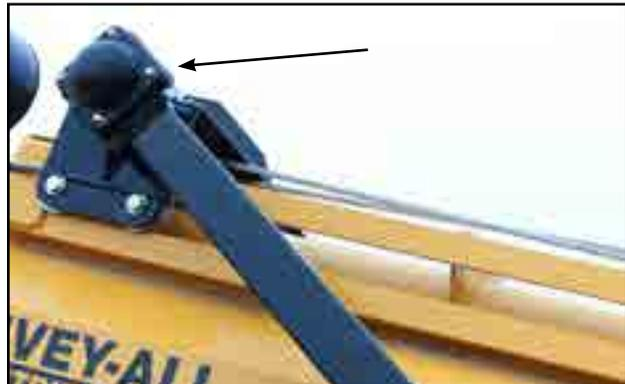
Fig 37 - Top slide bracket bearing
