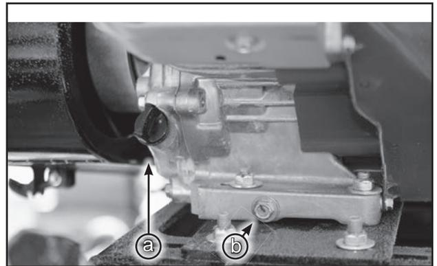
Fig 65 - Engine Oil - Fill Plug (a) and Drain Plug (b)
