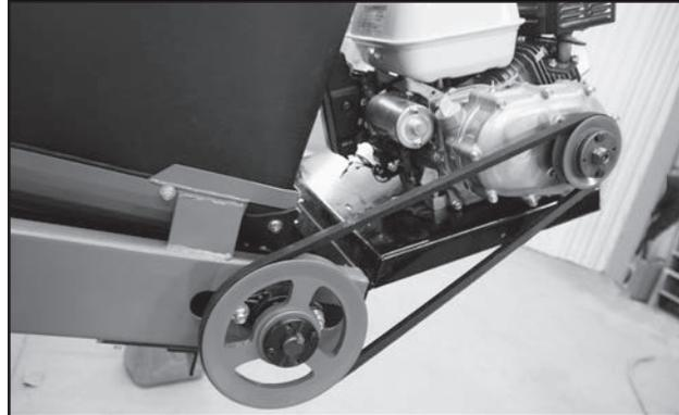
Fig 44 - Drive Belt, Guard Removed
