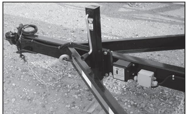
Fig 17 - Hitch, Jack, Breakaway System, Electrical Box
