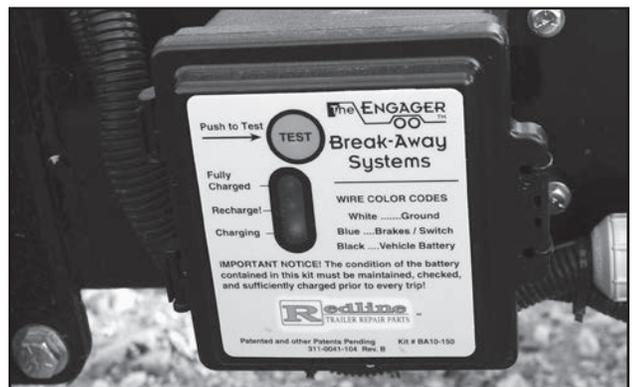
Fig 18 - Breakaway Switch Control Box
