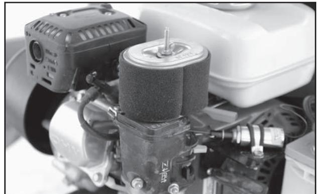
Fig 50 - Air Filter, Cover Removed
