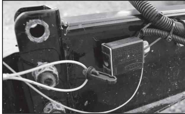
Fig 19 - Break-Away Switch with Pin Removed
