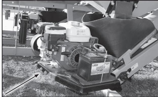
Fig 6 - Engine Mount Bolts
