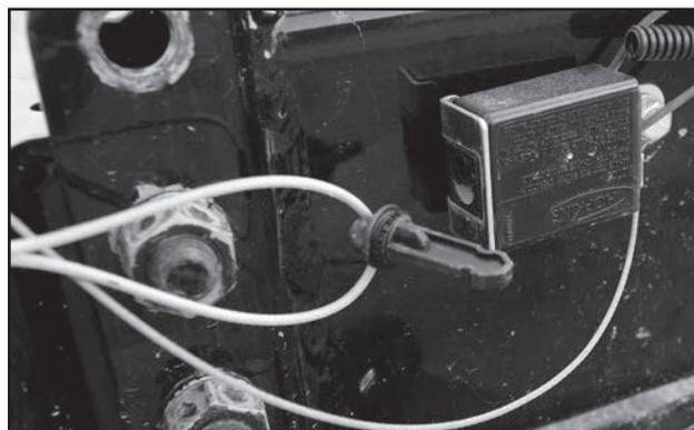
Fig 47 - Break-Away Switch Pin
