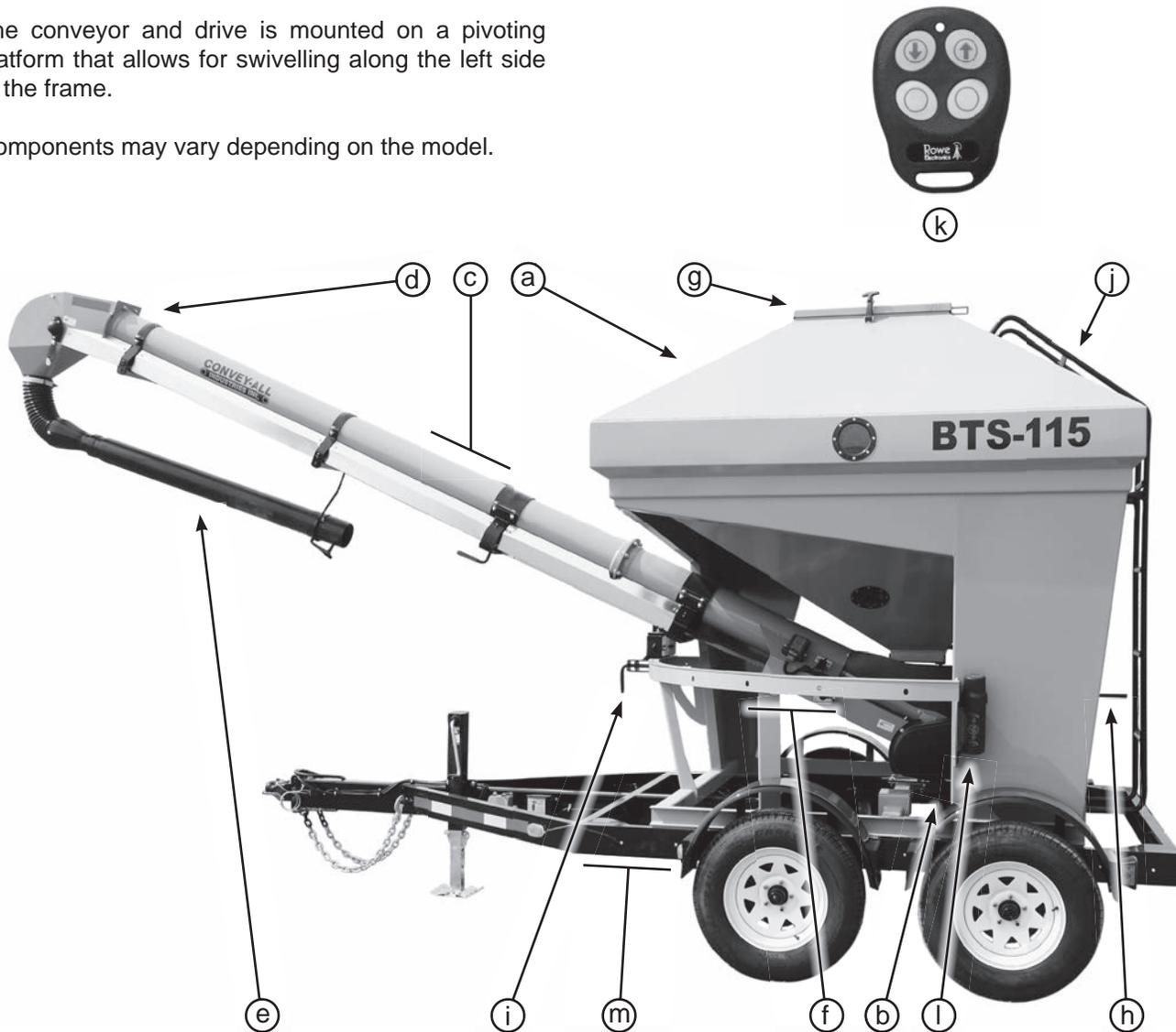
Fig 3 - BTS-115 and Remote Control Fob
