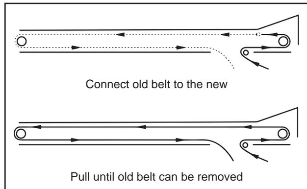
Fig 58 - Threading the Belt
