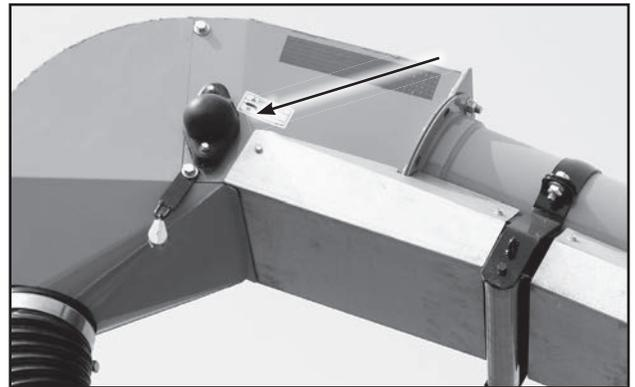
Fig 41 - Discharge Roller Bearing
