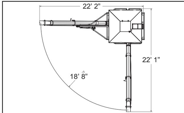
Fig 7 - Conveyor Pivot Schematic
