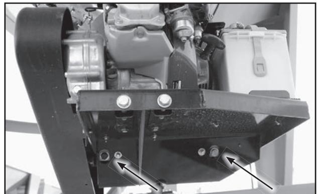
Fig 43 - Conveyor Tension Bolts
