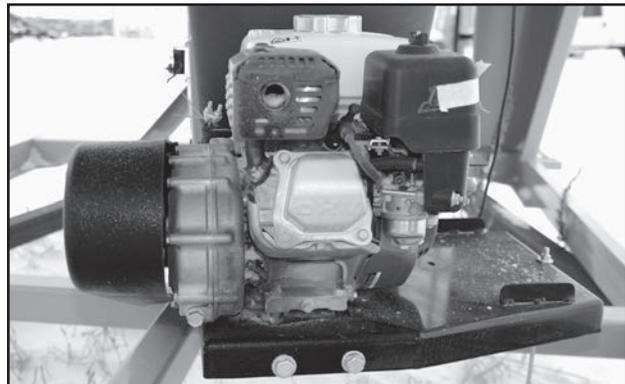
Fig 31 - Engine with Centrifugal Clutch
