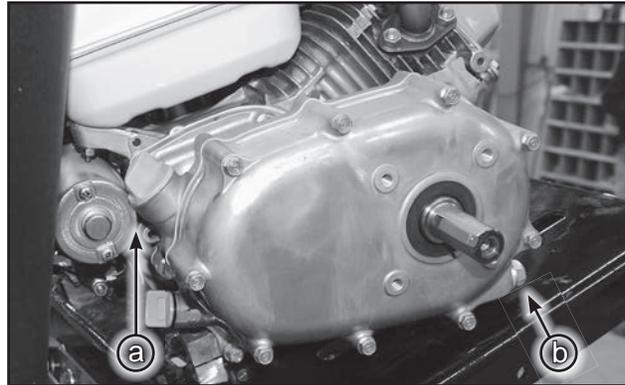
Fig 67 - Centrifugal Clutch - Fill Plug (a) and Drain Plug (b)
