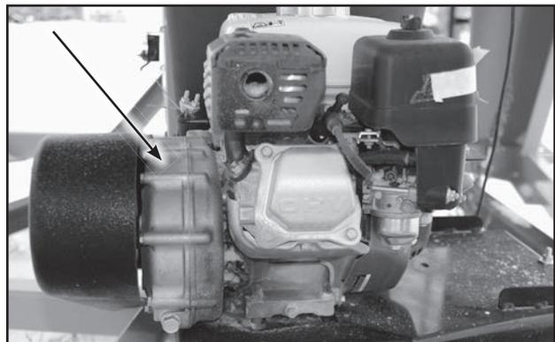
Fig 39 - Centrifugal Clutch
