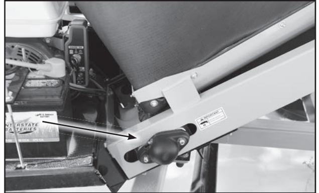
Fig 40 - Hopper Roller Bearing
