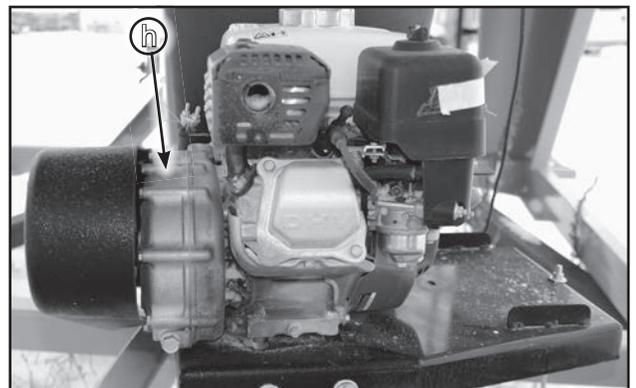
Fig 5 - Centrifugal Clutch
