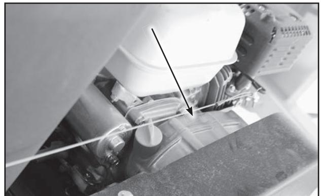
Fig 51 - Centrifugal Clutch
