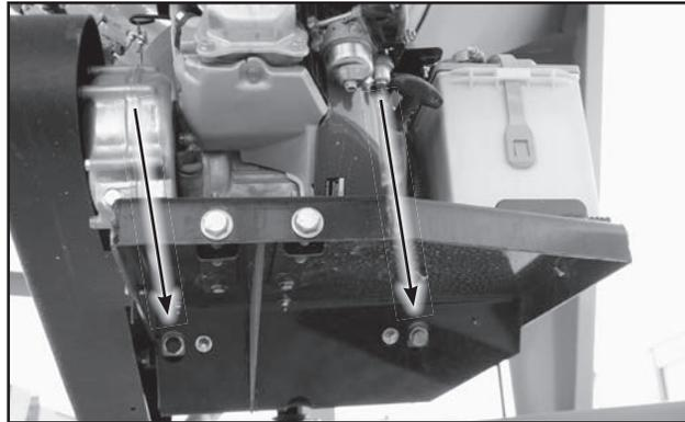
Fig 53 - Tension Bolts, Below Engine
