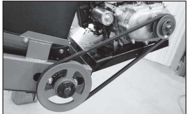
Fig 60 - Drive Belt, Guard Removed
