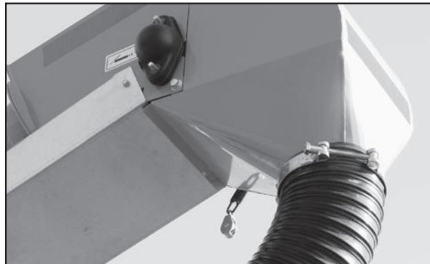
Fig 24 - Down Spout Fastened to Discharge
