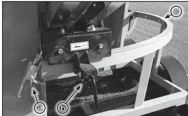
Fig 8 - Transport Lock (a), Roller Bracket Pin (b), Hole (c)
