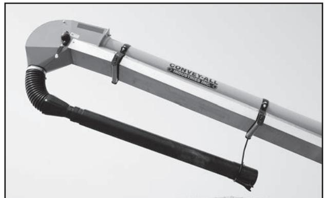
Fig 13 - Discharge Spout with Extension
