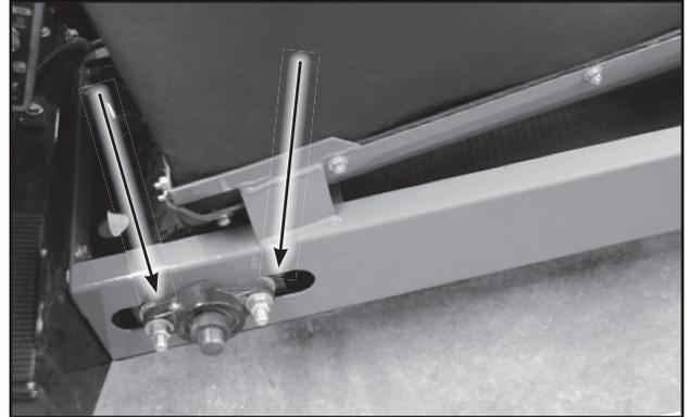
Fig 54 - Roller Bearing Anchor Bolts, Guard Removed
