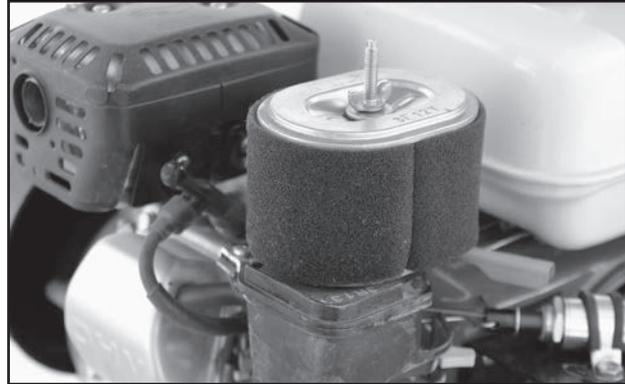
Fig 66 - Air Filter with Cover Removed
