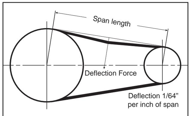
Fig 62 - Tension Calculation
