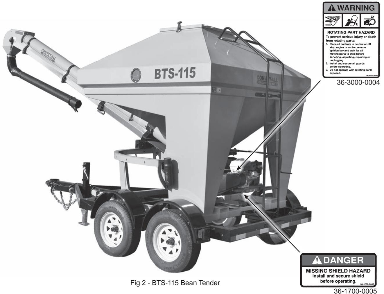
**REMEMBER** - If safety decals have been damaged, removed, become illegible, or parts were replaced without signage, new decals must be applied. Decals are available from your authorized dealer.
