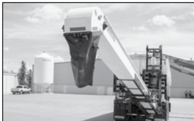
Fig 21 - Folding conveyor discharge spout
