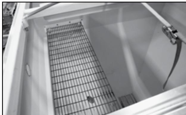
Fig 16 - Hopper catwalk
