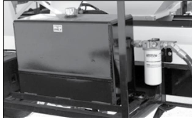
Fig 59 - Hydraulic reservoir and filter
