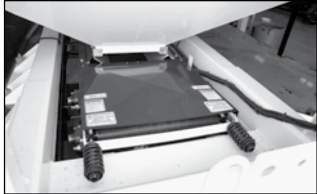
Fig 63 - Tension bolt on slave conveyor
