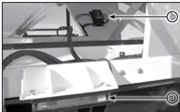
Fig 18 - Weight scale load cell
