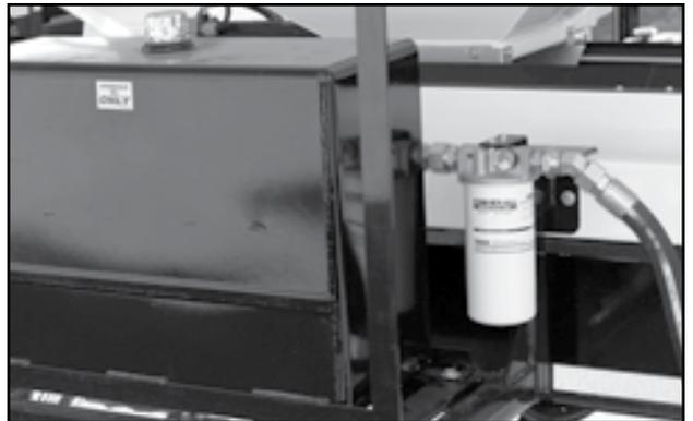
Fig 57 - Hydraulic system oil filter
