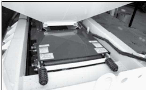
Fig 60 - Slave conveyor tension bolt and springs
