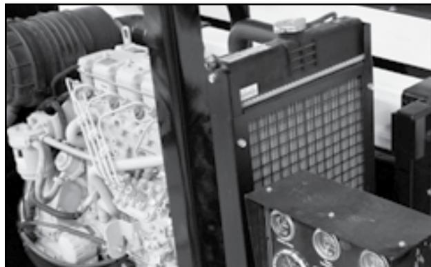
Fig 47 - Diesel engine
