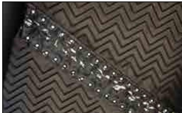
Fig 39 - Super screw® lacing
