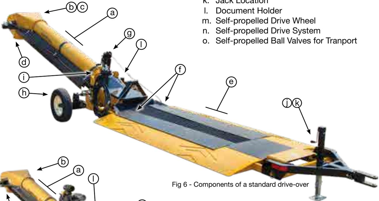
Fig 6 - Components of a standard drive-over
