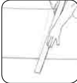
Cut your belt with a 1/3 bias (or 10% min of the width of the belt). The other side of the belt should be cut with a bias in the opposite direction.
