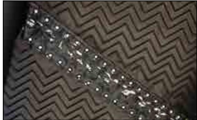
Fig 63 - Super-screw® lacing
