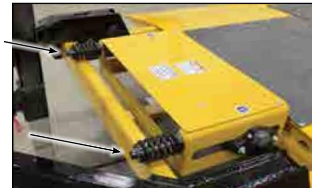
Fig 56 - Tail roller tension bolt
