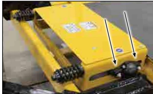
Fig 55 - Tail roller bearing anchor bolts
