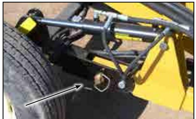
Fig 26 - Axle locking pin
