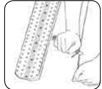
Chamfer the end of the belt top and bottom as shown. Position Super-Screw® against the belt, ensuring that Super-Screw® is resting against the central spacers.
