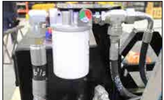
Fig 70 - Hydraulic oil filter
