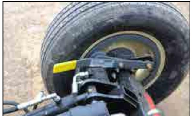
Fig 25 - Disengage drive wheel handle
