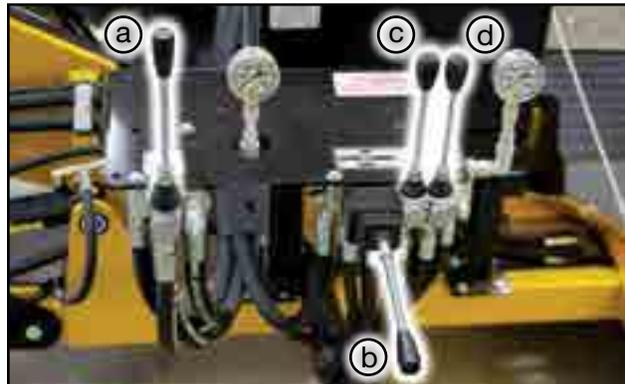
Fig 20 - Controls for self-propelled conveyor
