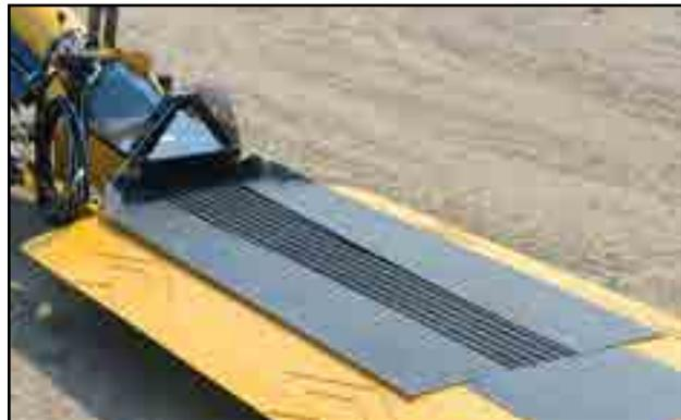
Fig 49 - Hopper flashing
