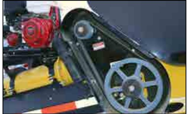
Fig 65 - Countershaft to belt roller belt
