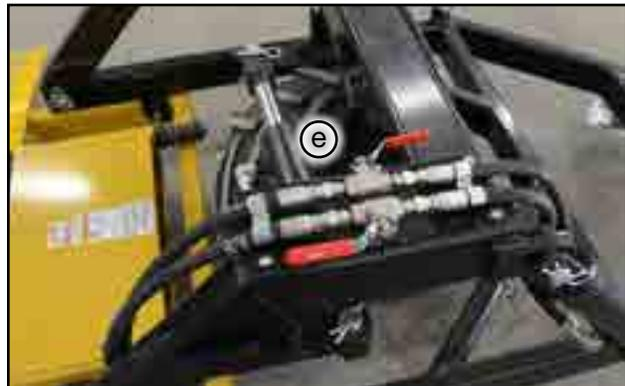
Fig 21 - Ball valves for transport
