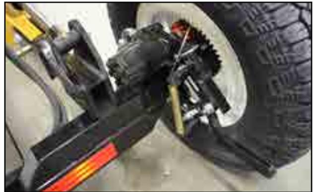
Fig 23 - Mover kit drive assembly - version 2
