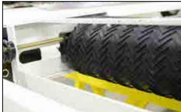
Fig 38 - Six Inch tail roller
