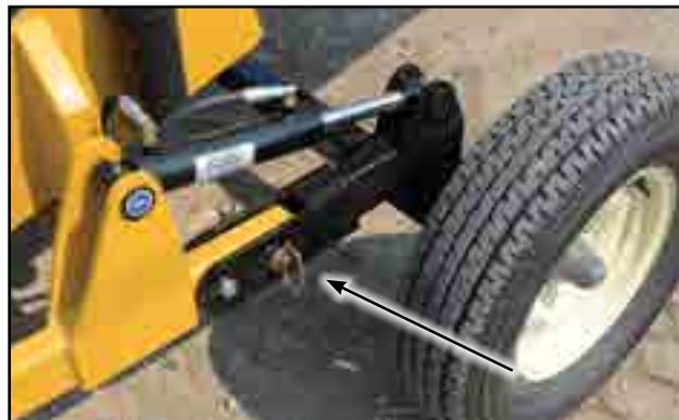
Fig 14 - Hydraulic cylinder on axle, and locking pin
