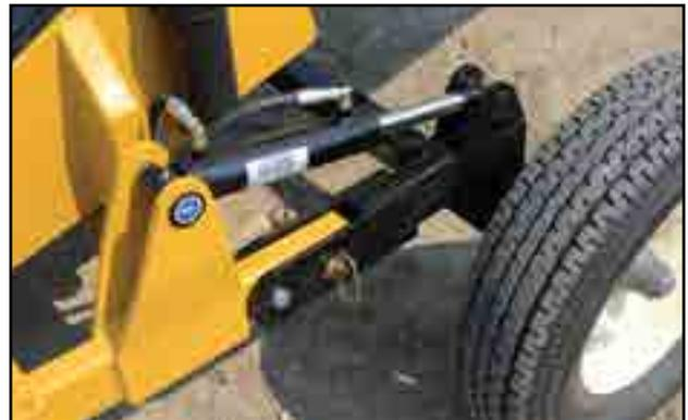
Fig 53 - wheel axle lift cylinders
