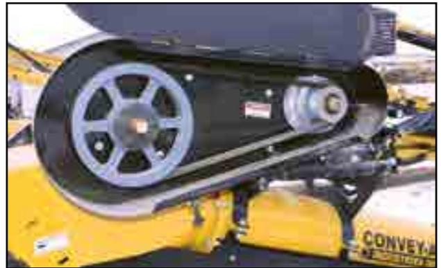
Fig 66 - Engine to countershaft
