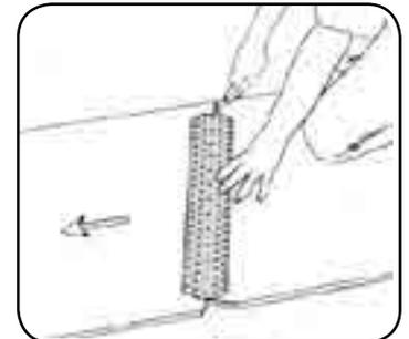
Cut the belt end (opposed to the trailing edge) as shown.
