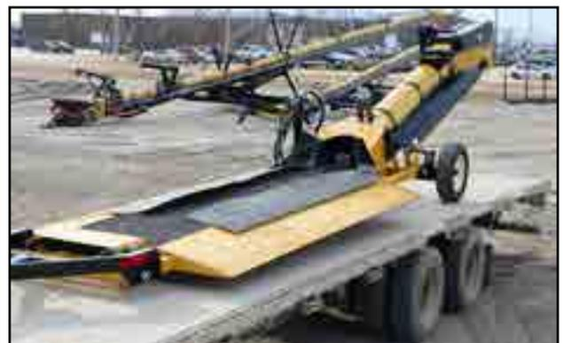
Fig 40 - Drive-over on a trailer
