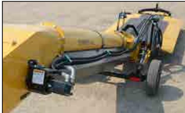
Fig 12 - Hydraulic motor
