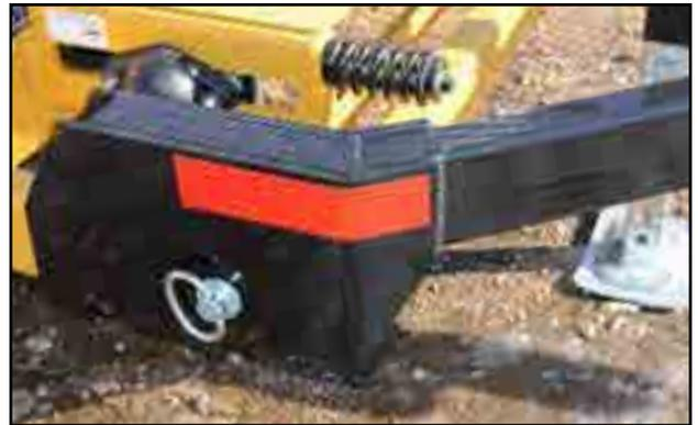
Fig 24 - Hitch anchor pins
