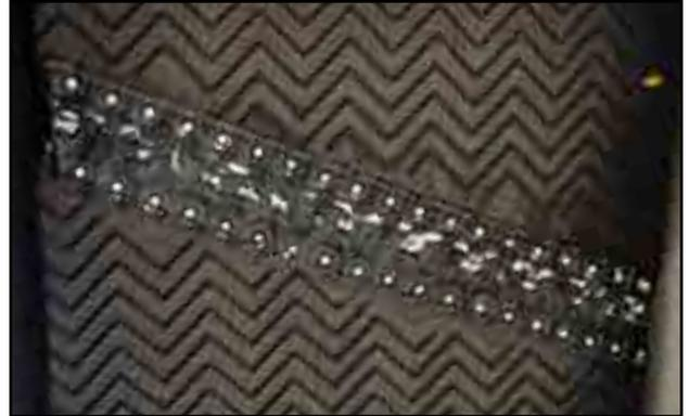
Fig 62 - Super-screw<sup>®</sup> lacing
