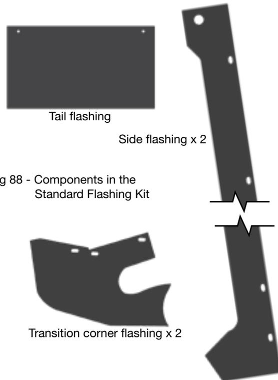
Fig 88 - Components in the Standard Flashing Kit
