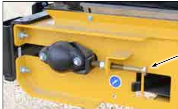
Fig 56 - Adjustment bolt on idler roller
