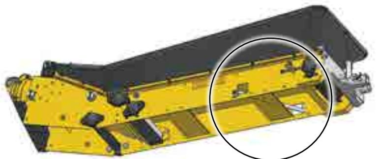
Fig 33 - Belt Scraper inside hopper frame
