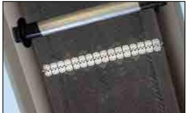
Fig 21 - Skived chevron belt with Alligator® lacing
