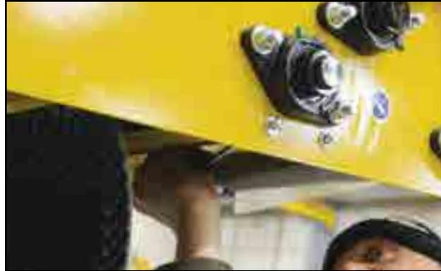
Fig 83 - Reinstall the containment plate
