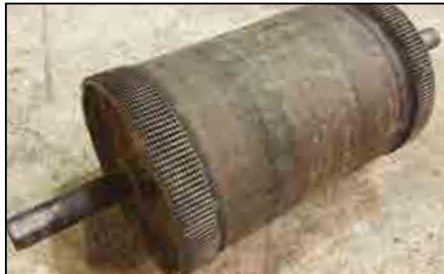
Fig 115 - Worn out drive roller
