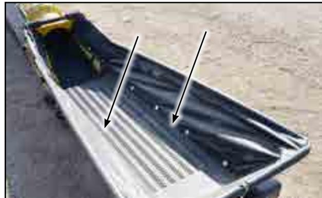
Fig 57 - Hopper flashing
