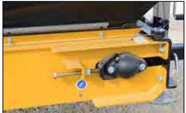
Fig 74 - Adjustment bolt at hopper idler roller
