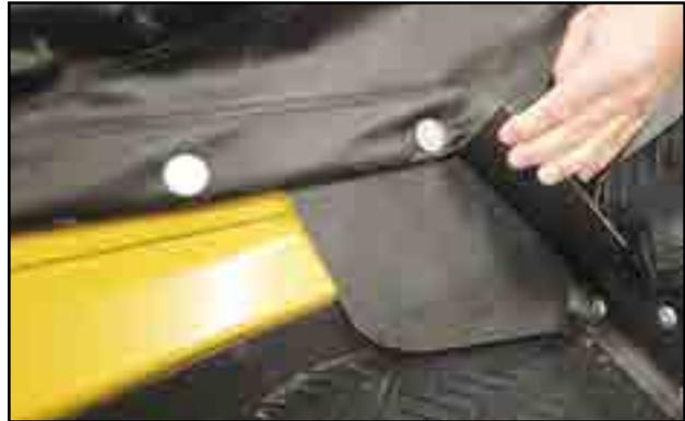
Fig 104 - Flashing fastened along transition
