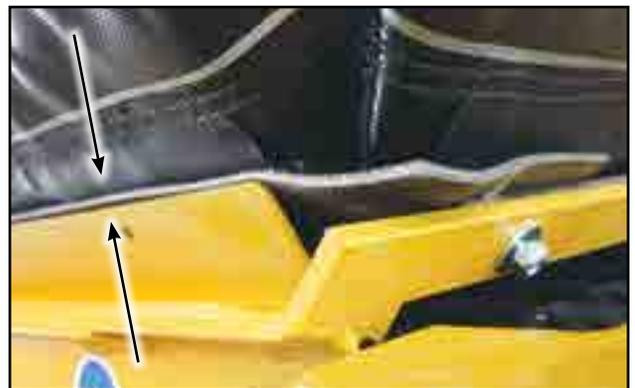
Fig 101 - Flashing flush with brackets
