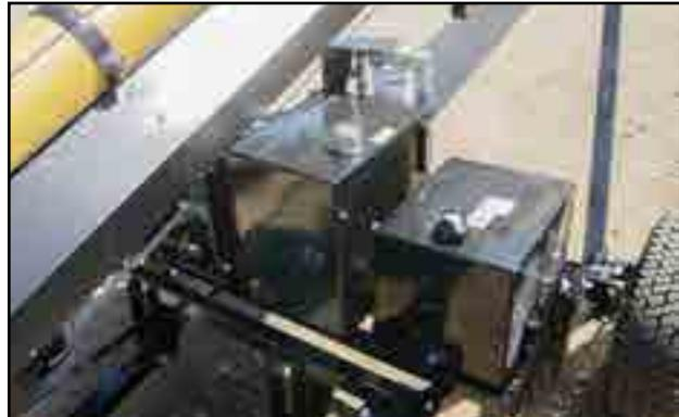
Fig 12 - Fuel tank and hydraulic reservoir
