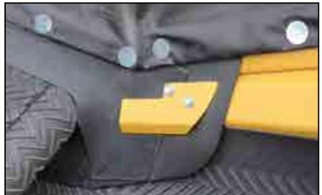
Fig 94 - Fasten flashing clamp
