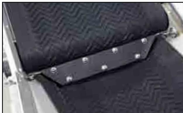
Fig 98 - Transition Flashing in place
