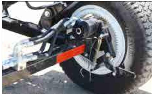
Fig 47 - Disengage drive wheels
