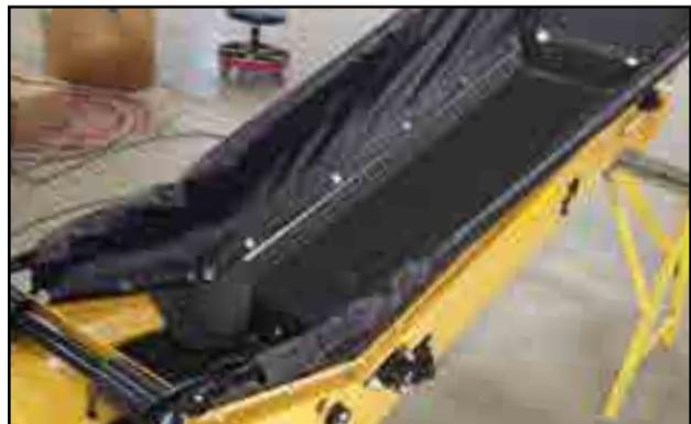
Fig 107 - Rubber flashing install
