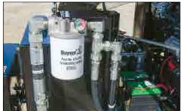
Fig 86 - Hydraulic Oil Filter
