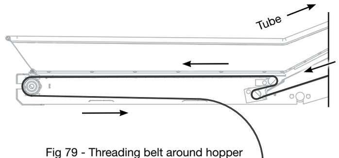
Fig 79 - Threading belt around hopper
