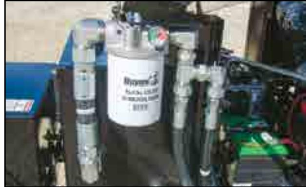
Fig 63 - Hydraulic filter
