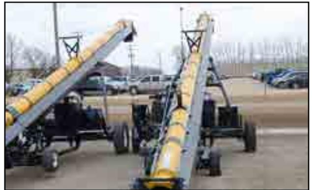
Fig 68 - Straight conveyor tube
