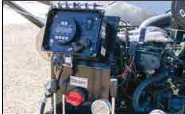
Fig 11 - Diesel engine control box
