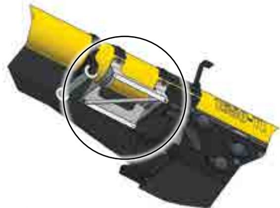
Fig 32 - Scraper before the drive box
