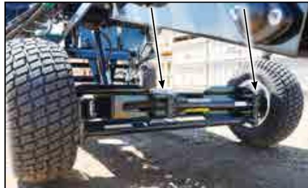
Fig 64 - Steering wheel axle bushings
