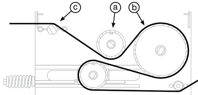
Fig 76 - 5" pinch roller (a), 10" drive roller (b), idler roller (c)
