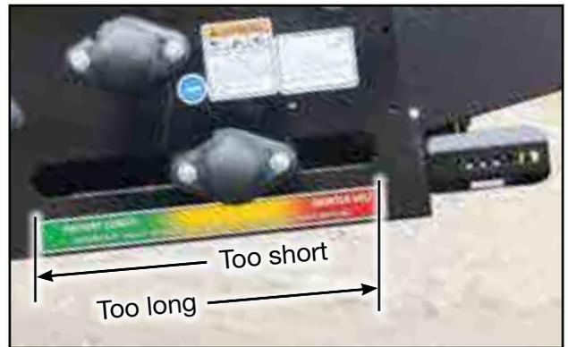
Fig 46 - “Slack Eliminator” roller. Belt length indication
