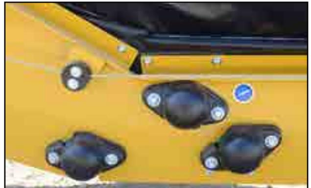
Fig 60 - Transition roller bearings
