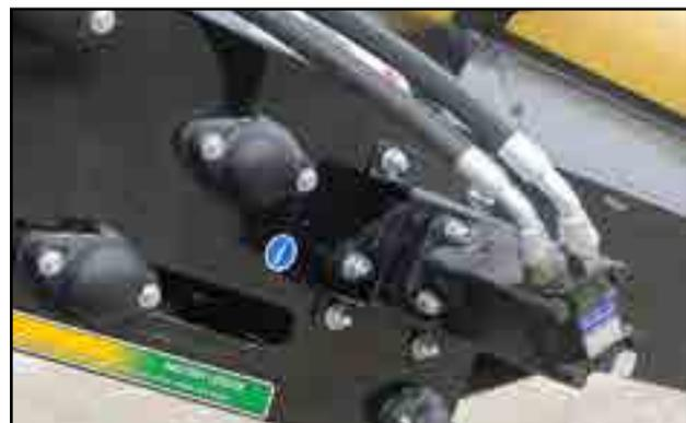
Fig 58 - Conveyor belt hydraulic drive motor
