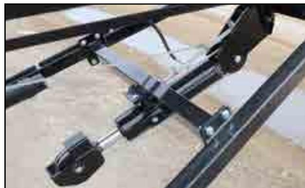
Fig 66 - Conveyor lift cylinder
