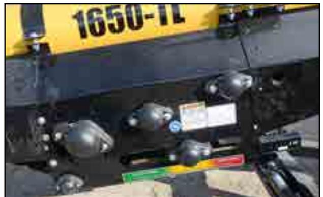
Fig 54 - Drive box roller bearings
