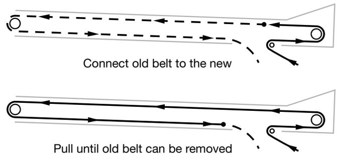
Fig 82 - Thread belt through conveyor
