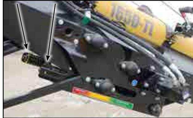
Fig 55 - Spring tension bolts, below drive box
