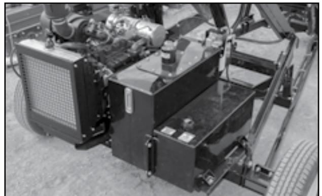
Fig 9 - Hydraulic oil reservoir and fuel tank
