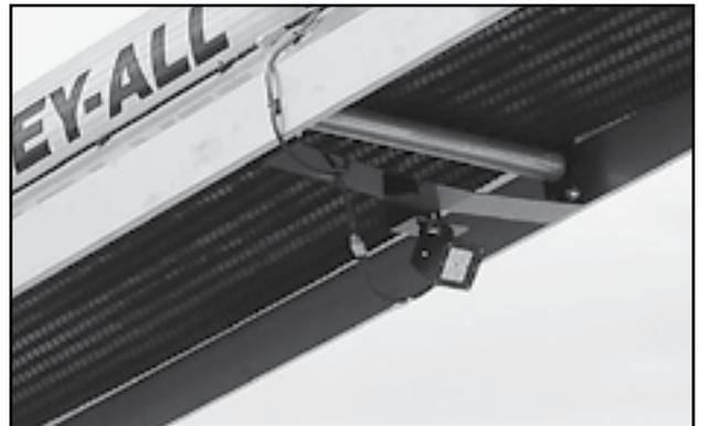
Fig 23 - Discharge working light
