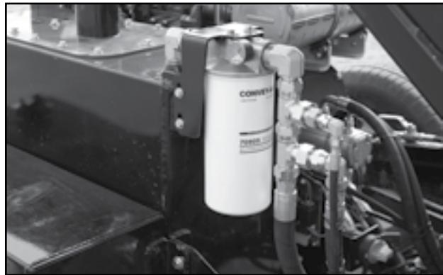
Fig 80 - Hydraulic Oil Filter
