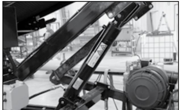
Fig 62 - Conveyor tube lift cylinder
