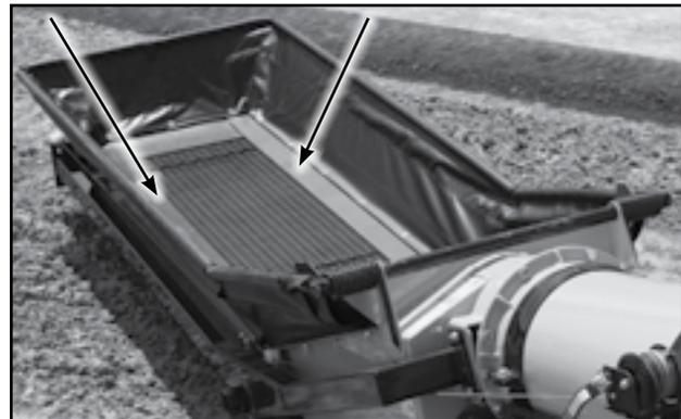
Fig 50 - Hopper flashing
