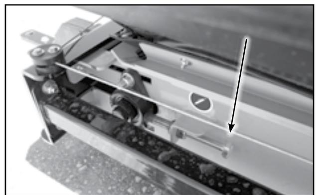
Fig 66 - Adjustment bolt at idler roller
