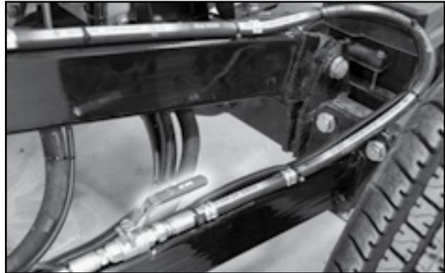
Fig 34 - Hydraulic ball valve to tube lift cylinder
