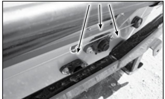
Fig 53 - Transition roller bearings
