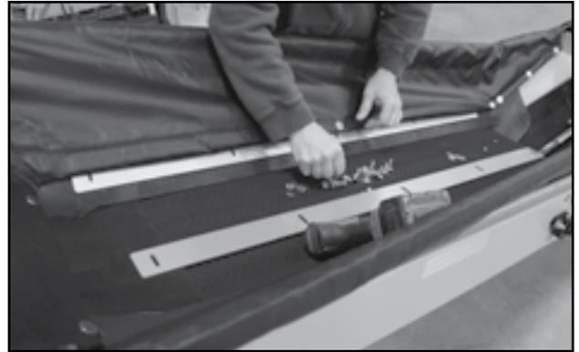
Fig 76 - Stainless steel flat bar to hold side flashing
