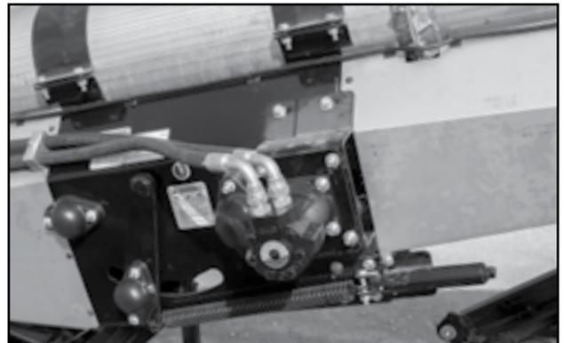
Fig 15 - Hydraulic Motor on Drive Box
