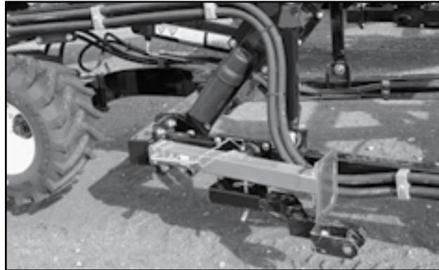
Fig 40 - Hitch and jack storage plate
