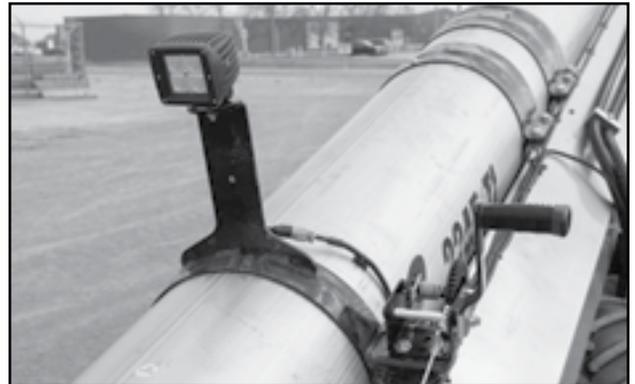
Fig 22 - Hopper working light
