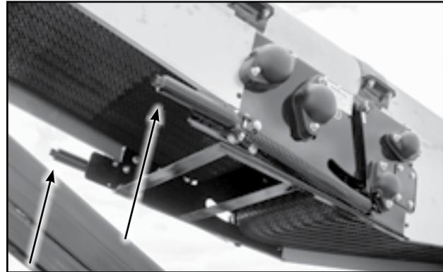
Fig 49 - Positive pinch drive tension bolts
