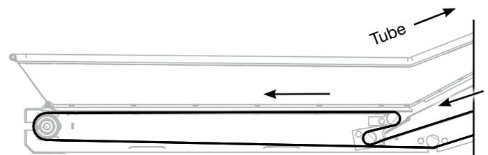
Fig 70 - Threading belt around hopper
