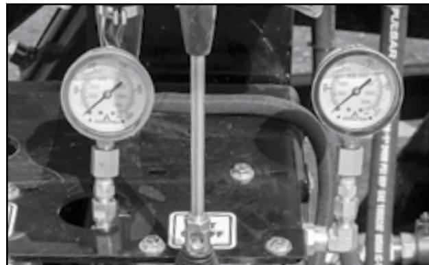
Fig 11 - Hydraulic pressure gauges
