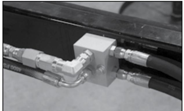
Fig 14 - Hydraulic manifold to drive wheel lift cylinder
