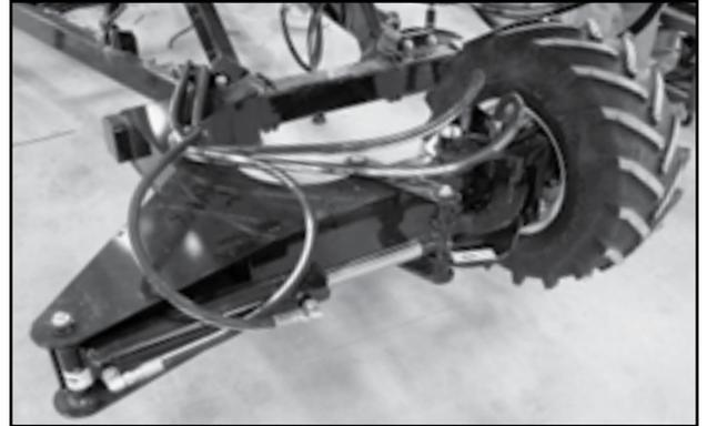
Fig 60 - Steering cylinder
