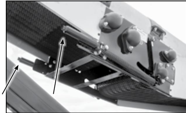
Fig 64 - Tension bolt
