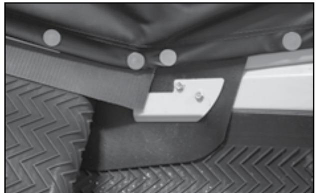
Fig 78 - Fasten flashing clamp
