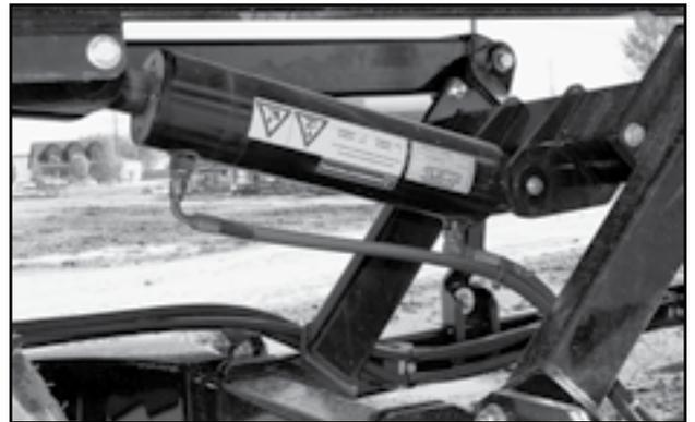
Fig 61 - Drive wheel lift cylinder
