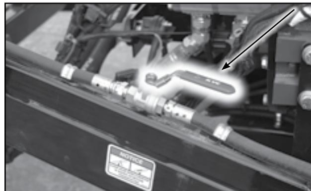
Fig 12 - Hydraulic ball valve to the lift cylinder
