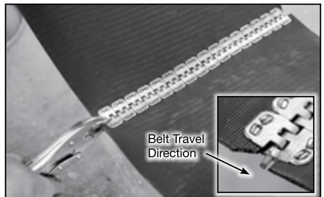
Fig 71 - Crimp lacing and taper belt corner
