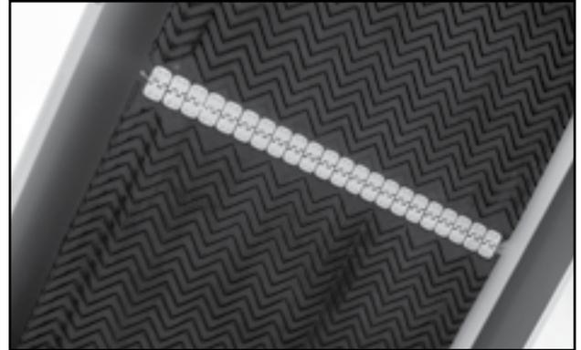
Fig 69 - Conveyor belt lacing
