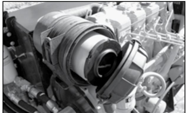
Fig 47 - Air filter with cover removed
