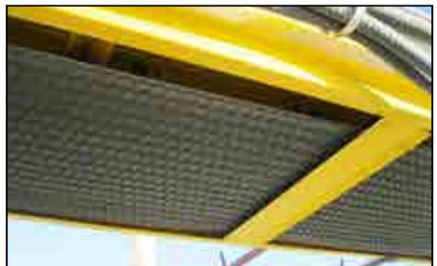
Fig 22 - Belt is inside bed frame
