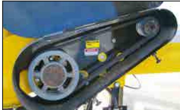
Fig 58 - Drive side with guard opened
