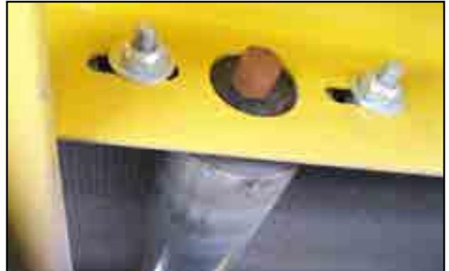
Fig 34 - Rollers are adjustable
