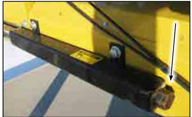
Fig 53 - End drive tensioning jacks
