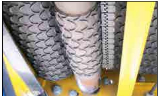
Fig 21 - Belt between discharge and drive roller
