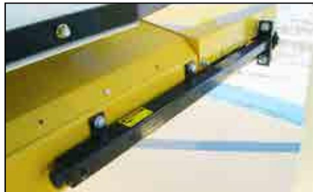
Fig 26 - Tensioning jacks on end drive system
