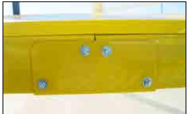
Fig 13 - Bed bolt plate
