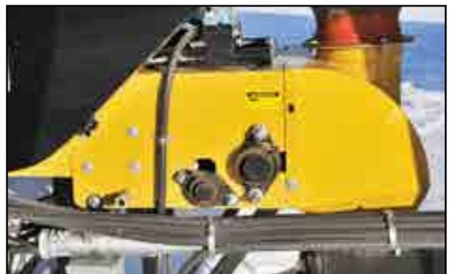
Fig 48 - Discharge and drive roller bearings
