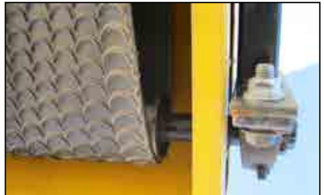
Fig 47 - Tail roller from underneath
