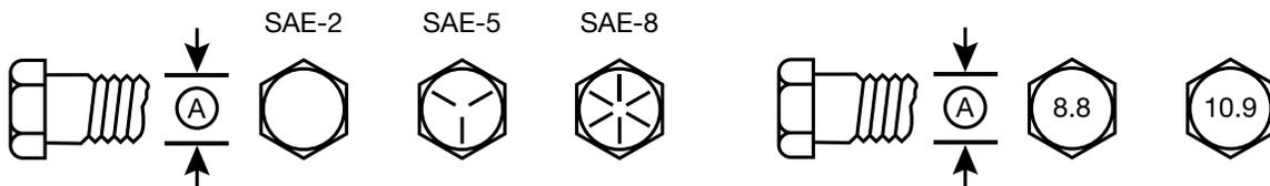
Torque figures indicated above are valid for non-greased or non-oiled threads and heads unless otherwise specified. Therefore, do not grease or oil bolts or capscrews unless otherwise specified in this manual. When using locking elements, increase torque values by 5%.
