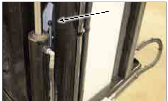
Fig 61 - Tension bolts on rear conveyor
