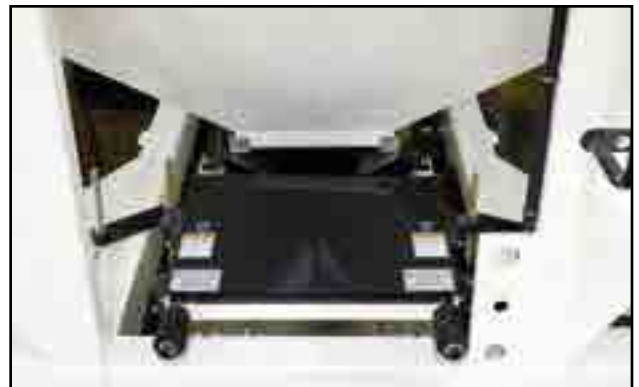
Fig 60 - Slave conveyor tension bolt and springs
