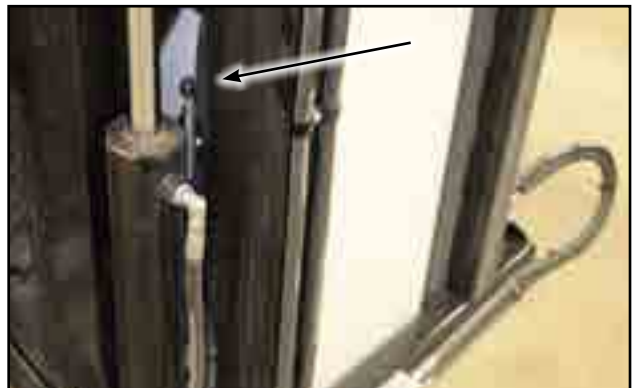
Fig 54 - Tension bolts on rear, fold conveyor
