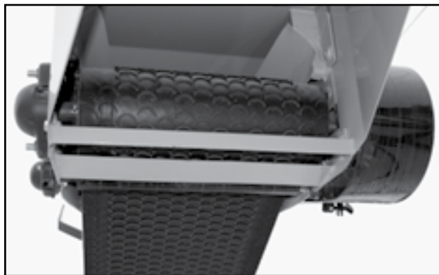
Fig 37 - Belt aligned in discharge hood
