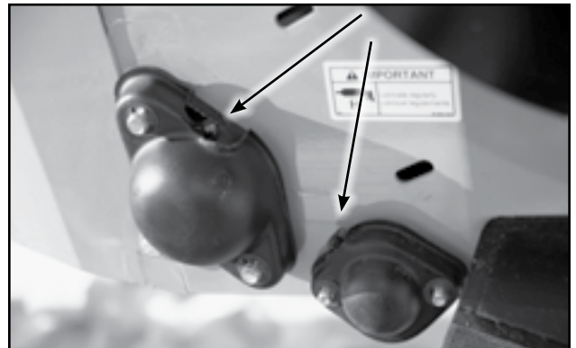
Fig 43 - Discharge Roller Bearings Zerk
