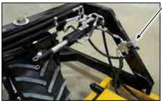
Fig 24 - Mover kit steering wheel hydraulics and solenoid
