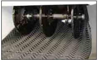
Fig 38 - Hold-down wheel transition
