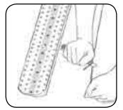
Chamfer the end of the belt top and bottom as shown. Position Super-Screw® against the belt, ensuring that Super-Screw® is resting against the central spacers.
