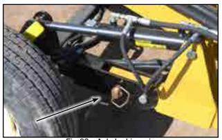
Fig 22 - Axle locking pin
