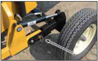
Fig 14 - Hydraulic cylinder on axle, and locking pin
