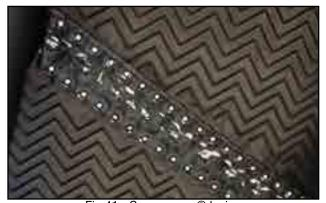
Fig 41 - Super screw® lacing
