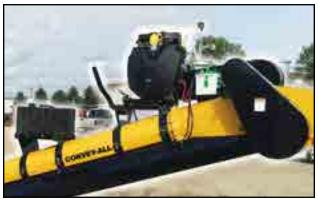
Fig 8 - Gas engine mounted on tube
