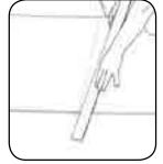
Cut your belt with a 1/3 bias (or 10% min of the width of the belt). The other side of the belt should be cut with a bias in the opposite direction.
