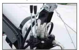
Fig 13 - Hydraulic valves
