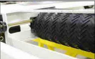
Fig 40 - Six Inch tail roller
