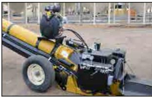
Fig 19 - Mover kit engine, drive wheels and hydraulics
