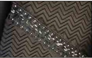
Fig 65 - Super-screw® lacing
