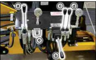
Fig 20 - Controls for self-propelled conveyor
