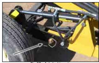
Fig 27 - Axle locking pin
