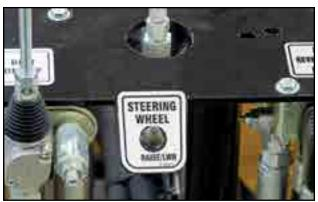
Fig 23 - Steering wheel toggle switch
