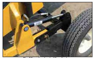
Fig 55 - wheel axle lift cylinders
