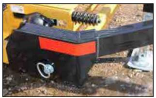
Fig 25 - Hitch anchor pins
