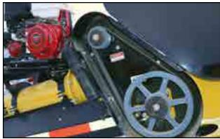
Fig 67 - Countershaft to belt roller belt
