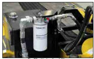
Fig 72 - Hydraulic oil filter
