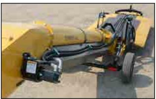
Fig 12 - Hydraulic motor
