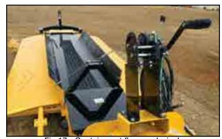
Fig 17 - Containment flaps and winch
