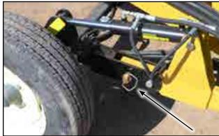
Fig 42 - Axle locking pin
