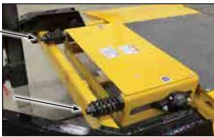
Fig 58 - Tail roller tension bolt
