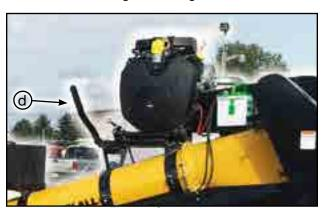
Fig 10 - Gas engine
