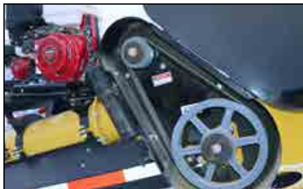
Fig 58 - Countershaft to drive roller V-belt
