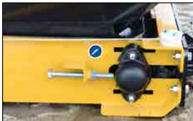
Fig 48 - Roller bearing mounts and anchor bolts
