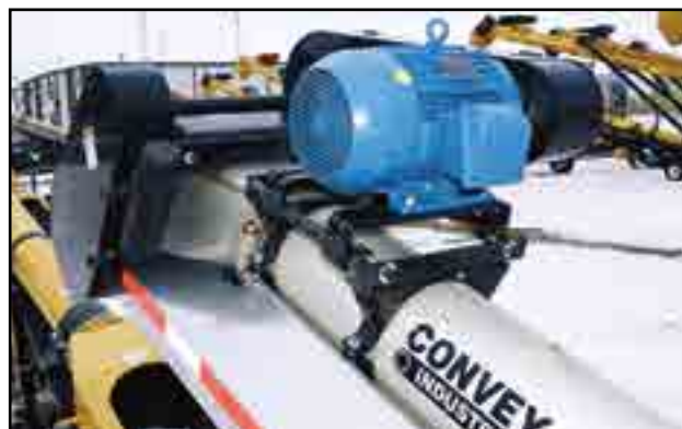
Fig 61 - Electric motor, speed reduction drive
