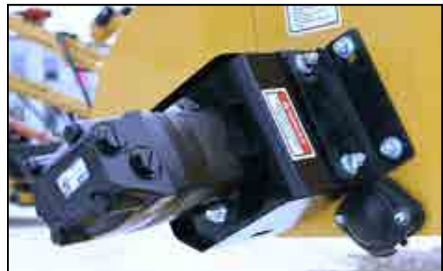
Fig 8 - Hydraulic motor, hoses not attached
