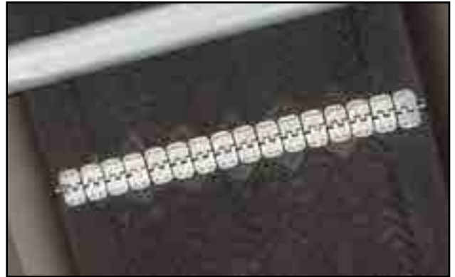
Fig 9 - Chevron belt with Alligator® lacing
