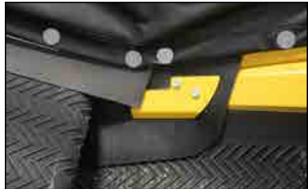
Fig 68 - Fasten flashing clamp
