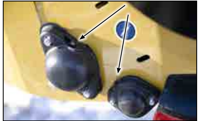
Fig 40 - Bearing grease zerks
