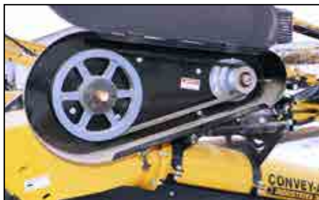
Fig 59 - Engine to countershaft V-belt
