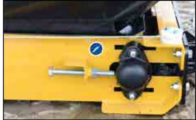
Fig 37 - Hopper roller bearing
