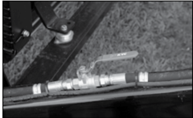
Fig 52 - Hydraulic ball valve to tube lift cylinder
