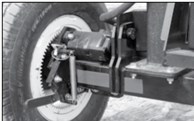
Fig 105 - Wheel ring gear and drive motor
