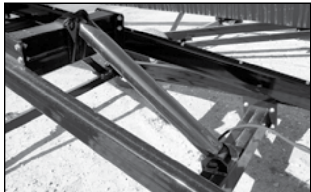
Fig 75 - Conveyor tube lift cylinder
