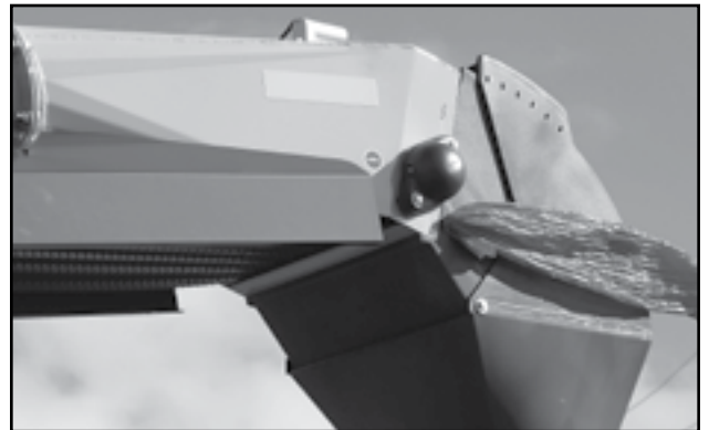
Fig 70 - discharge roller bearing
