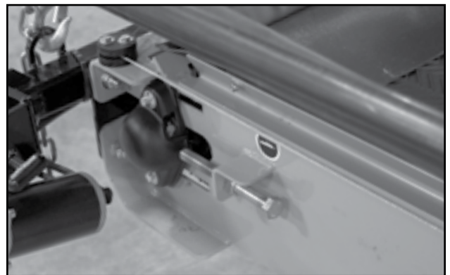
Fig 81 - Swing-out hopper roller bearing
