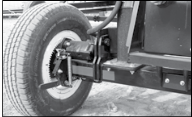
Fig 102 - Bin fill conveyor drive wheel
