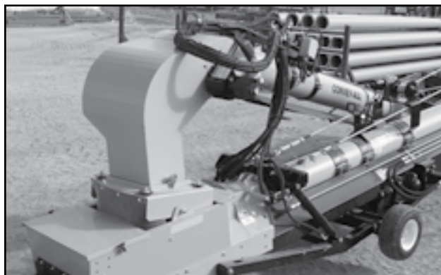
Fig 34 - Discharge of swing-out with manual winch
