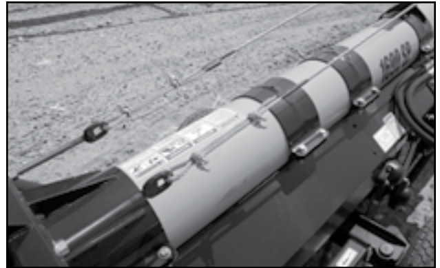
Fig 76 - Eyebolts and cable bridging
