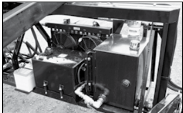
Fig 11 - Fuel tank and hydraulic reservoir
