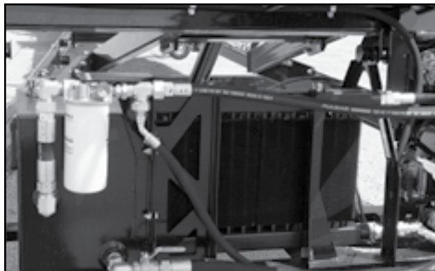
Fig 12 - Hydraulic Filter and Hydraulic Cooler
