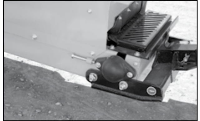
Fig 68 - Adjustment bolts on side of hopper
