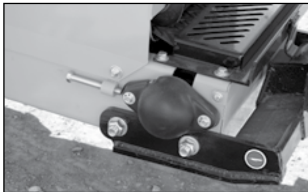
Fig 63 - Hopper roller bearings
