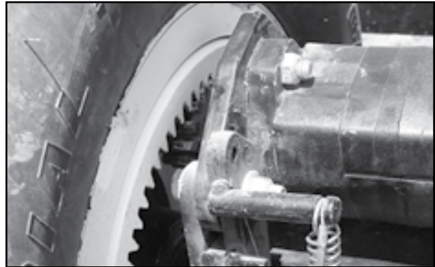
Fig 103 - Bin fill conveyor drive gears
