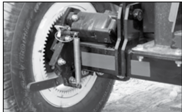
Fig 67 - Sprockets on drive wheel
