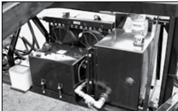
Fig 61 - Hydraulic oil reservoir and fuel tank
