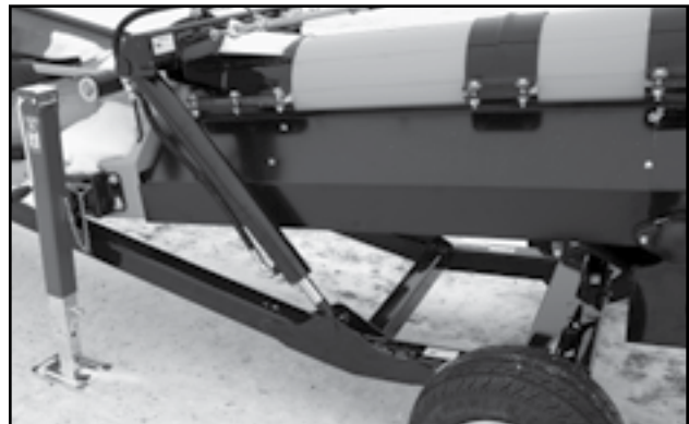
Fig 74 - Steering wheel lift cylinder
