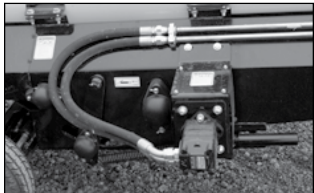
Fig 18 - Drive box with hydraulic motor
