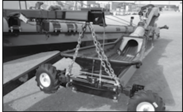
Fig 37 - Swing-out with electric mover kit
