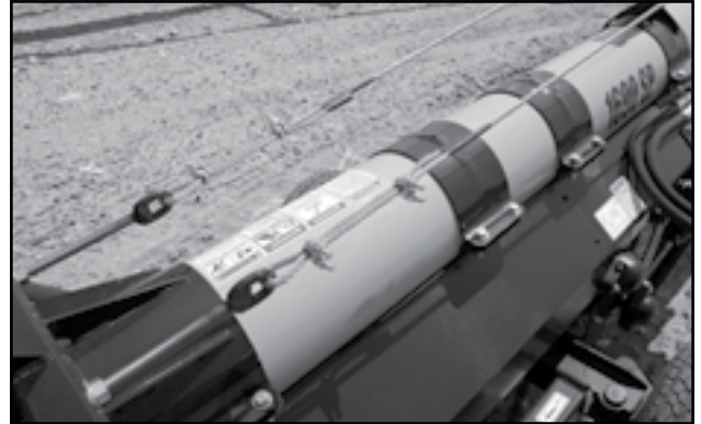
Fig 76 - Eyebolts and cable bridging
