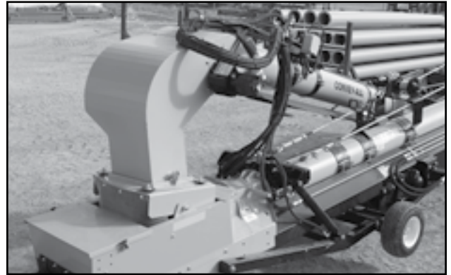
Fig 34 - Discharge of swing-out with manual winch
