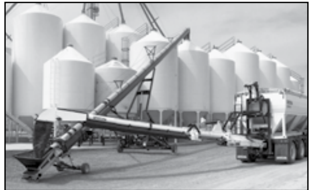
Fig 55 - CST unloading into conveyor
