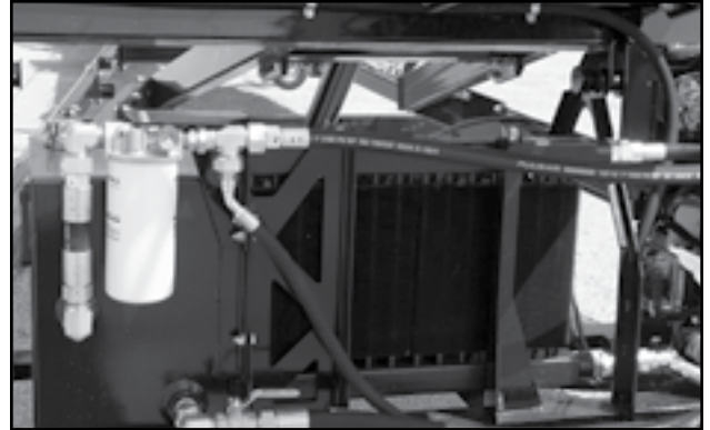
Fig 12 - Hydraulic Filter and Hydraulic Cooler
