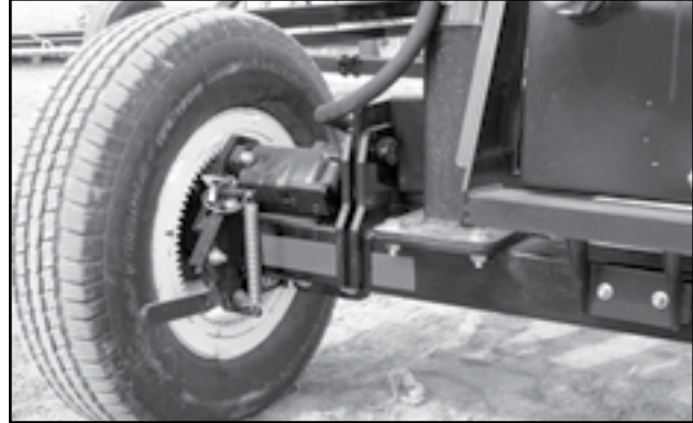
Fig 110 - Bin fill conveyor drive wheel
