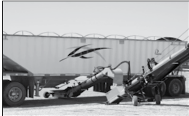
Fig 54 - Trailer unloading into swing-out conveyor
