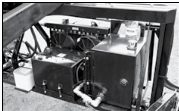
Fig 11 - Fuel tank and hydraulic reservoir
