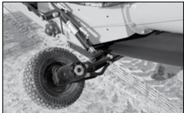
Fig 34 - Swing-out mover kit
