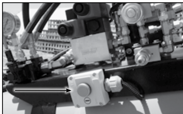
Fig 44 - Green, manual over-ride switch
