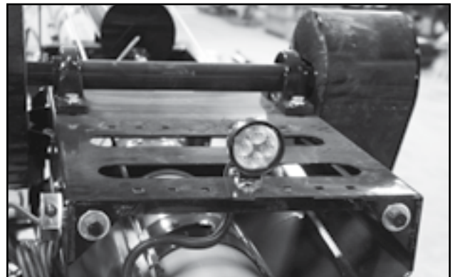
Fig 19 - Hopper working light
