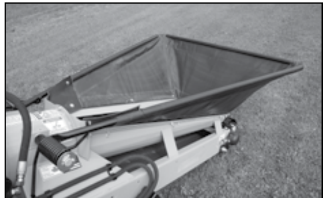
Fig 32 - Hopper on the ground
