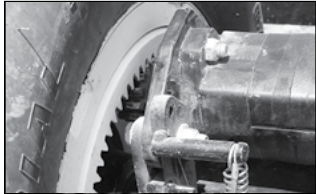
Fig 88 - Bin fill conveyor drive gears
