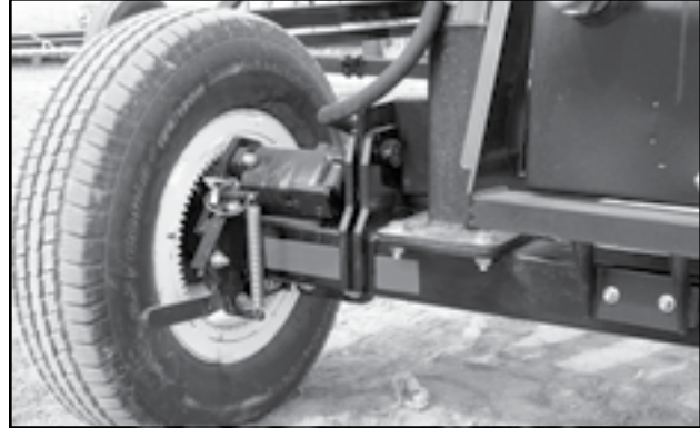
Fig 87 - Bin fill conveyor drive wheel
