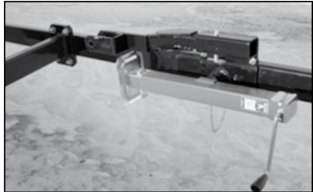
Fig 26 - Jack and drawbar in storage
