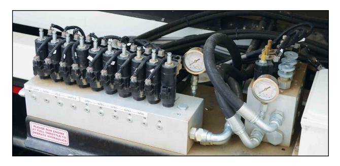
This type of valve block was installed on tenders manufactured between 2018 and 2019.
