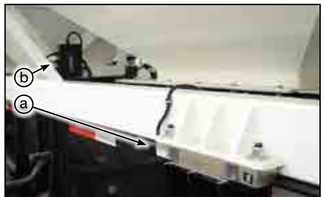
Fig 16 - (a) Load Cell, (b) weigh scale junction box
