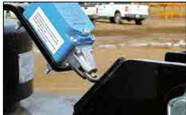
Fig 19 - Rotation centre limit switch
