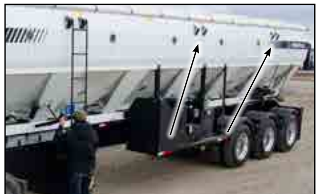
Fig 30 - Exterior ladder brackets
