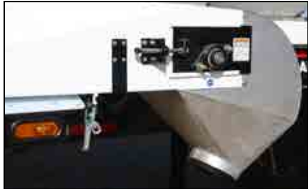
Fig 59 - Adjustment bolt, rear conveyor discharge
