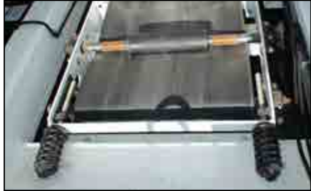
Fig 58 - Slave conveyor tension bolts, belt cover removed
