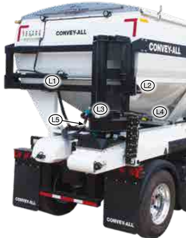
Fig 17 - Limit switches controlling rear conveyor movements
