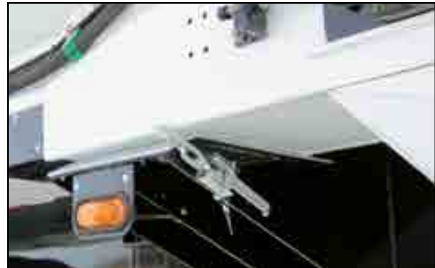
Fig 42 - Rear conveyor transport lock
