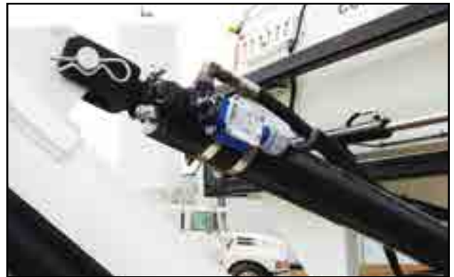
Fig 21 - Rotation centre limit switch
