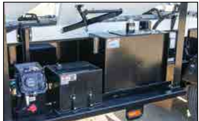
Fig 11 - Fuel tank and hydraulic oil reservoir
