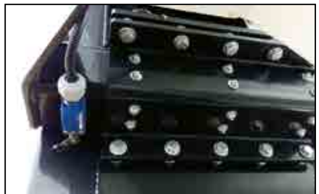
Fig 23 - Rotation centre limit switch
