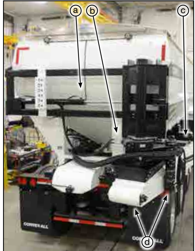
Fig 60 - Rear conveyor movement points
