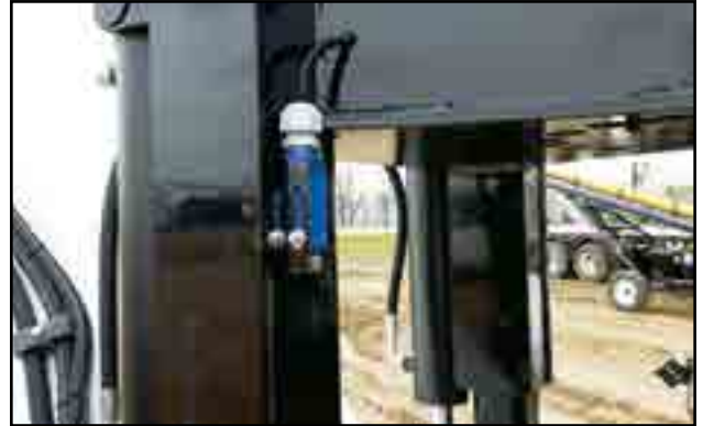
Fig 20 - Rotation centre limit switch
