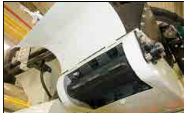
Fig 18 - Hopper access panel
