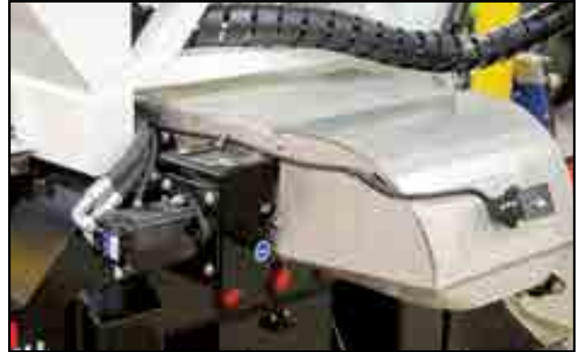
Fig 56 - Slave conveyor drive
