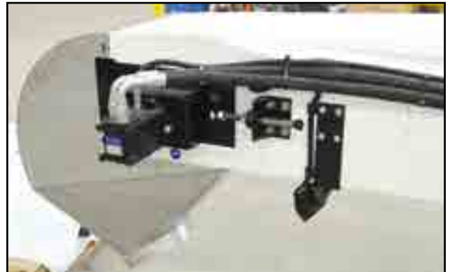
Fig 57 - Rear conveyor drive
