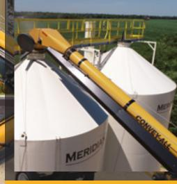
The 1600 Series uses a 16" belt inside a 10" tube, and is available in 35' to 100' lengths. They have a capacity of up to 6,000 bu/hr.
