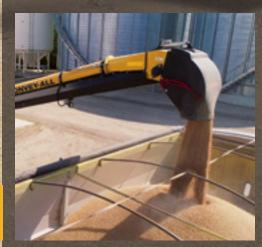
These conveyors are available with 16" or 22" belt widths. They are perfect for moving product from a bin, to a truck or trailer.
