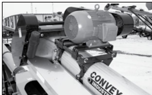
Fig 59 - Electric motor, speed reduction drive
