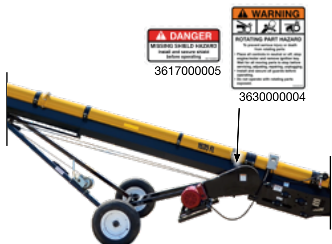
Fig 4 - Conveyor with electric drive
