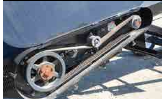
Fig 63 - Drive belt with guard opened
