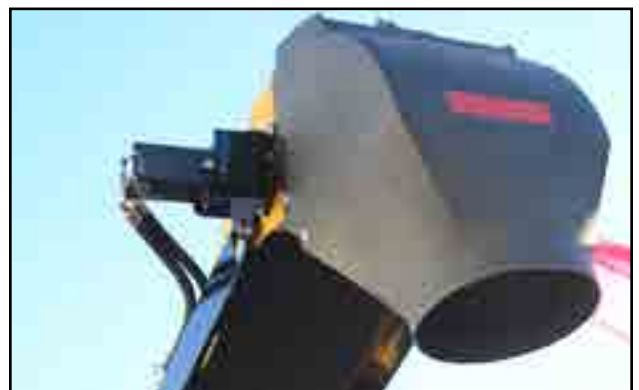
Fig 41 - Top-end hydraulic drive
