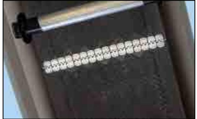
Fig 81 - Conveyor belt lacing
