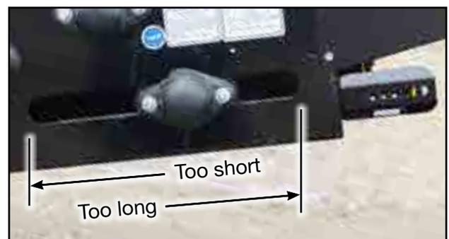
Fig 49 - “Slack Eliminator” roller. Belt length indication
