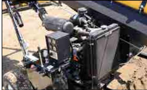
Fig 10 - Tier 4 diesel engine
