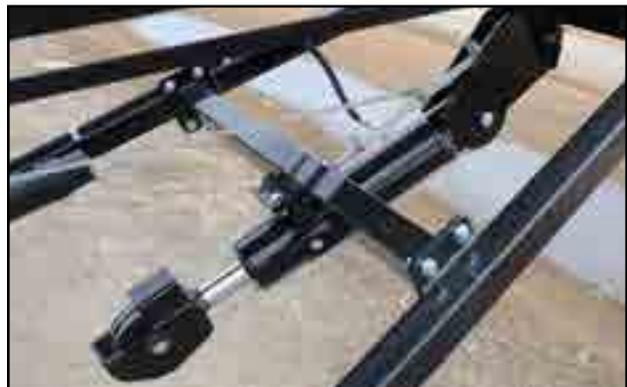
Fig 69 - Conveyor lift cylinder
