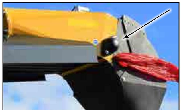
Fig 65 - Discharge roller bearing
