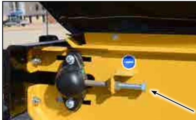
Fig 59 - Adjustment bolt on tail roller
