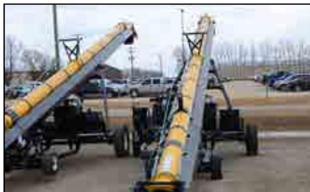
Fig 20 - Straight conveyor tube
