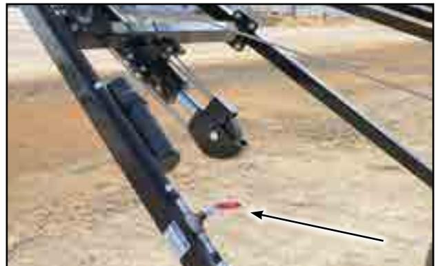
Fig 16 - Lift cylinder and ball valve
