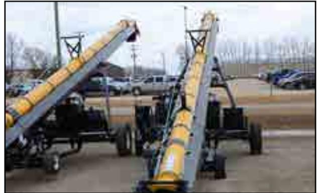
Fig 71 - Straight conveyor tube
