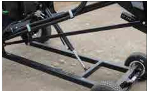
Fig 68 - Steering wheel lift cylinder
