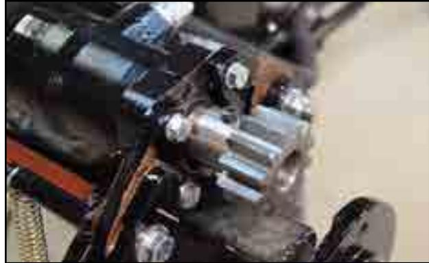
Fig 112 - Pinion gear
