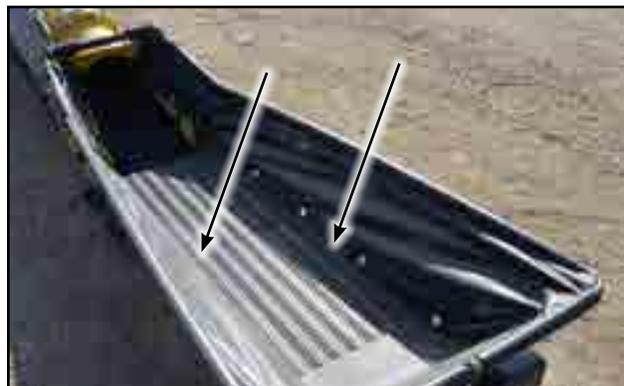
Fig 60 - Hopper flashing
