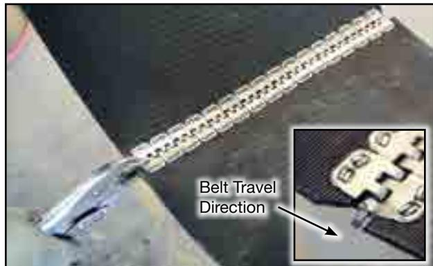
Fig 88 - Crimp lacing and taper belt corner
