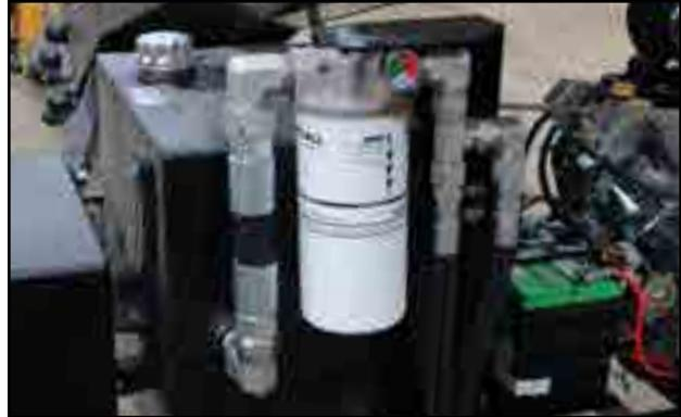
Fig 66 - Hydraulic filter
