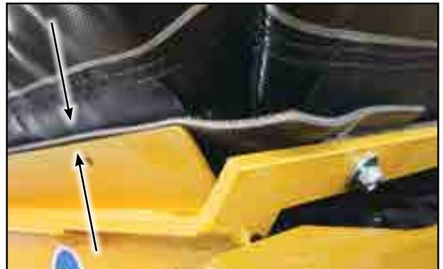
Fig 103 - Flashing flush with brackets
