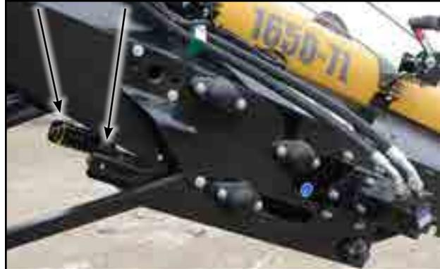
Fig 58 - Spring tension bolts, below drive box
