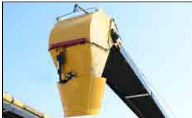
Fig 28 - Quad-swivel discharge spout and transport lights
