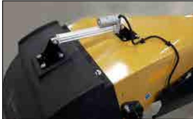
Fig 26 - Electric actuator
