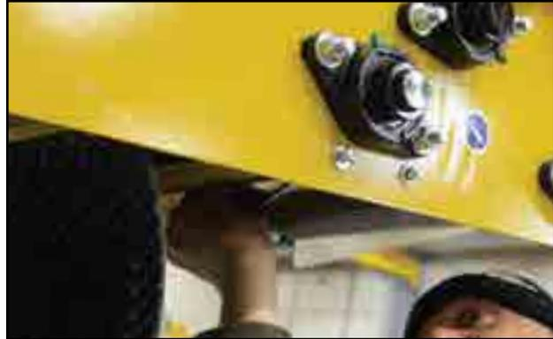
Fig 86 - Reinstall the containment plate
