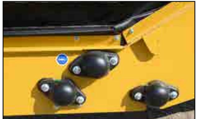
Fig 63 - Transition roller bearings
