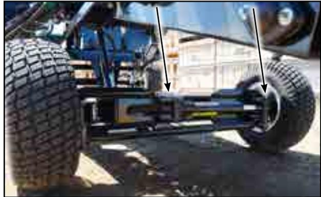
Fig 67 - Steering wheel axle bushings
