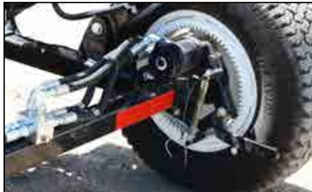
Fig 50 - Disengage drive wheels
