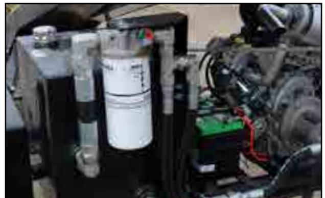
Fig 89 - Hydraulic Oil Filter
