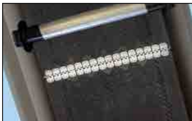
Fig 19 - Skived chevron belt with Alligator® lacing
