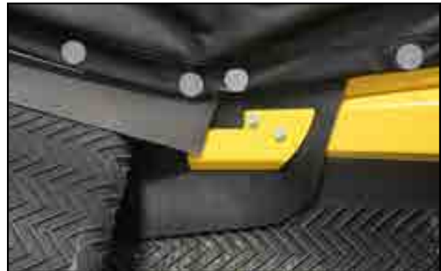
Fig 69 - Fasten flashing clamp
