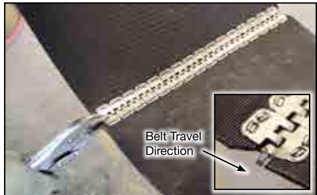
Fig 59 - Crimp lacing and taper belt corner
