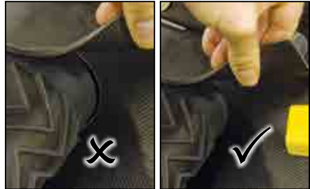
Fig 68 - Corner flashing must fit tight around the belt
