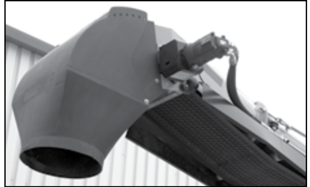
Fig 29 - Discharge spout with hydraulic drive
