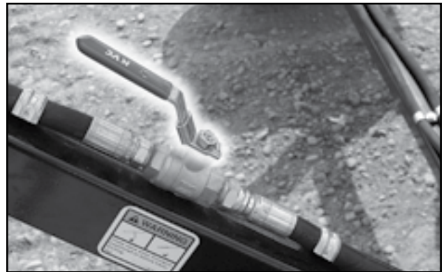
Fig 30 - Hydraulic ball valve to lift cylinder
