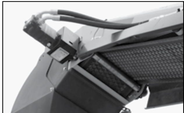
Fig 48 - Hydraulic motor, conveyor belt drive
