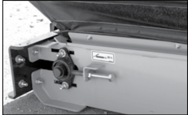
Fig 46 - Adjustment bolt on tail roller
