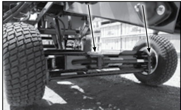
Fig 53 - Steering wheel axle bushings
