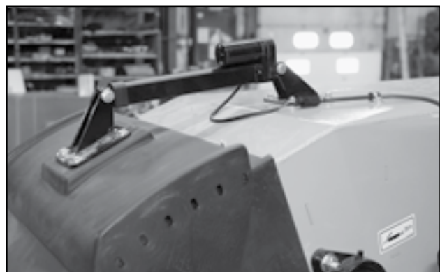
Fig 18 - Electric actuator on discharge spout
