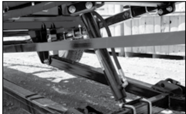
Fig 54 - Steering wheel lift cylinder
