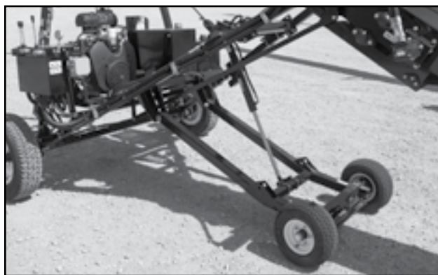
Fig 14 - Steering wheels with cylinder
