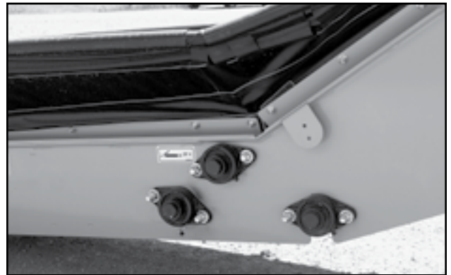
Fig 50 - Transition roller bearings
