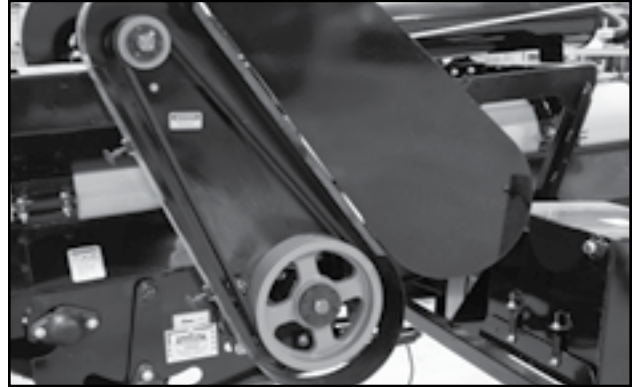
Fig 77 - Countershaft-to-Drive belt with guard open
