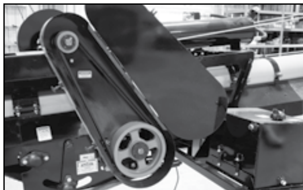
Fig 81 - Belt drive with guard opened
