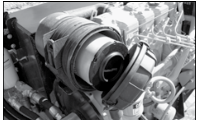
Fig 46 - Air filter with cover removed
