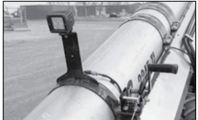
Fig 22 - Hopper working light
