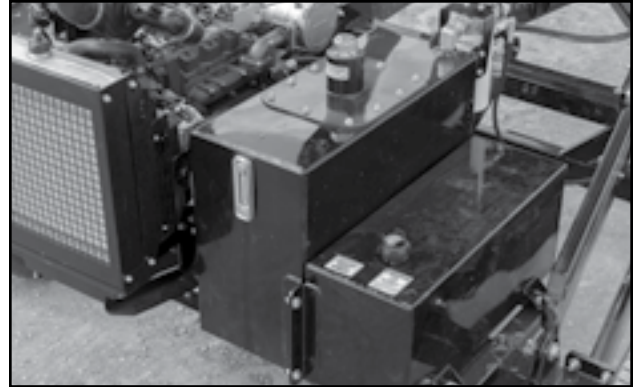
Fig 44 - Hydraulic oil reservoir and fuel tank
