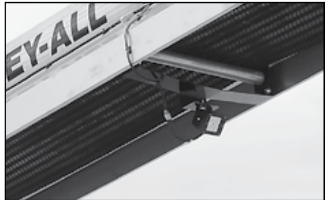
Fig 23 - Discharge working light
