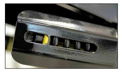
Outside both springs is an indicator window with integrated arrows, top and bottom.
