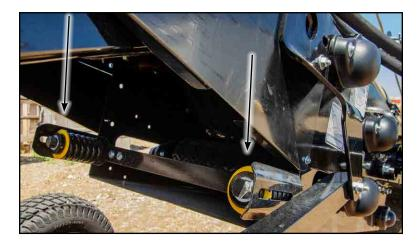
There is a yellow washer installed at the end of a spring on both sides of the belt, below the drive box.
