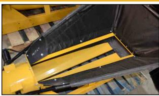
1. Install the Hopper Tail Flashing onto the front of the hopper, first.
