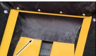
2. The Hopper Side Flashing must be placed over top the Tail Flashing.
