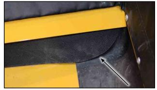
3. When the conveyor belt is threaded through the tube and hopper, be sure to pull it underneath the Side and Tail Flashing.
