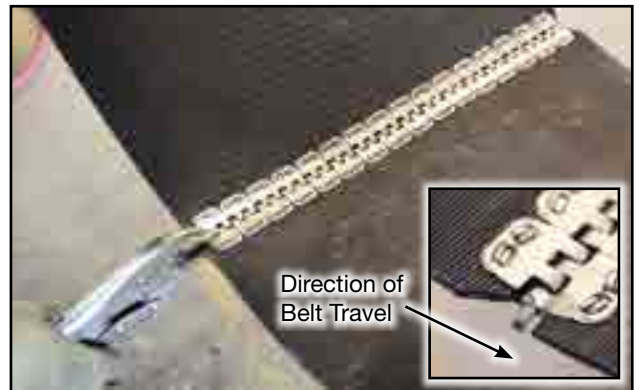
Fig 95 - Crimp lacing and taper belt corners
