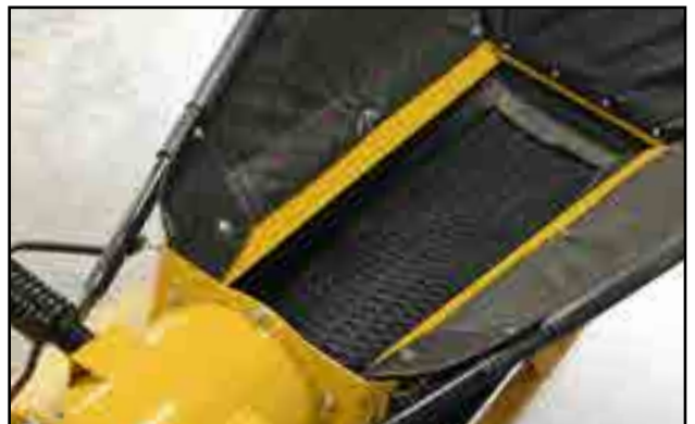
Fig 101 - Completed hopper with belt
