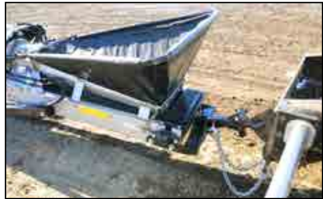
Fig 48 - Safety chain secured
