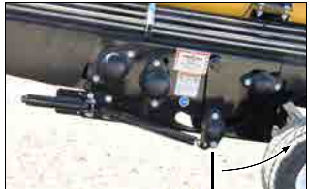
Fig 80 - Belt length indicator
