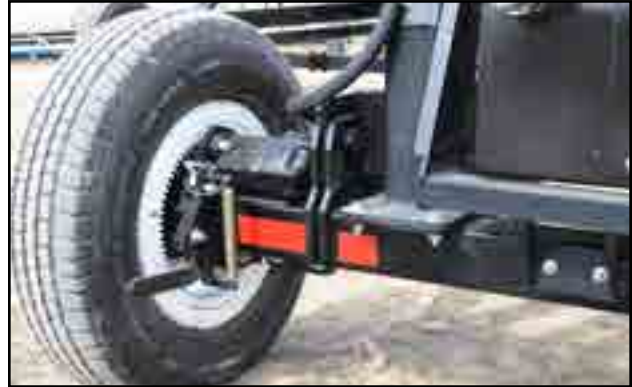
Fig 109 - Bin fill conveyor drive wheel
