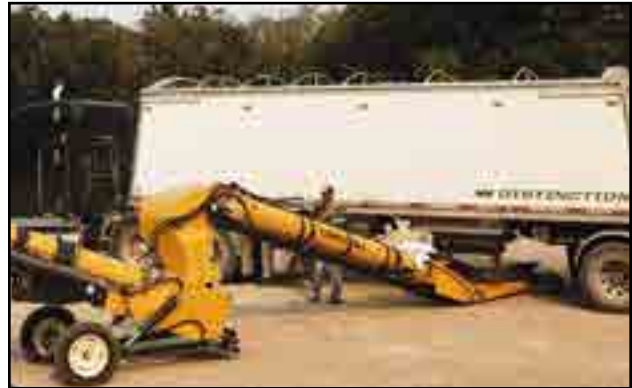
Fig 55 - Trailer unloading into swing-out conveyor
