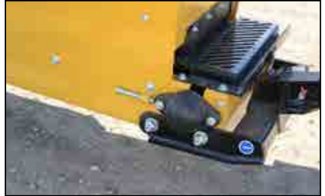
Fig 68 - Adjustment bolts on side of hopper
