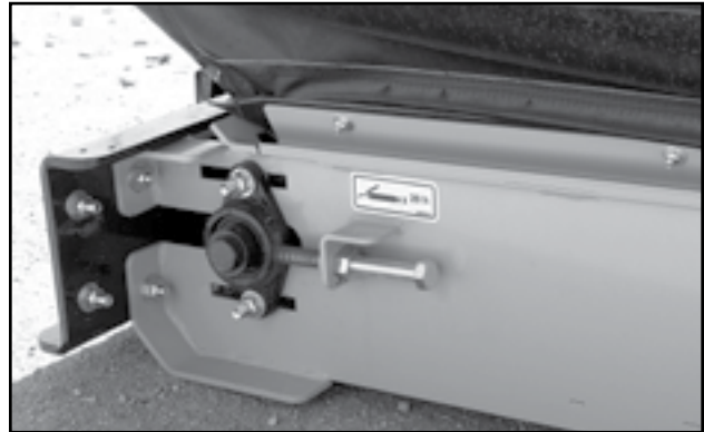
Fig 60 - Tail roller with adjustment bolt
