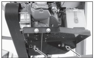
Fig 43 - Conveyor Tension Bolts
