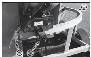
Fig 8 - Transport Lock (a), Roller Bracket Pin (b), Hole (c)
