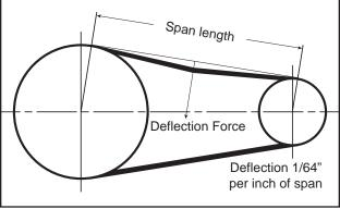
Fig 62 - Tension Calculation
