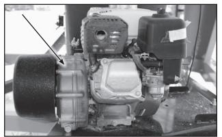
Fig 39 - Centrifugal Clutch
