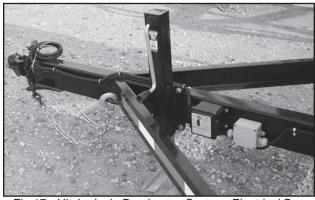
Fig 17 - Hitch, Jack, Breakaway System, Electrical Box
