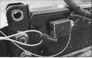
Fig 19 - Break-Away Switch with Pin Removed
