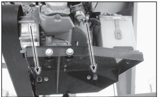
Fig 53 - Tension Bolts, Below Engine
