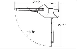
Fig 7 - Conveyor Pivot Schematic
