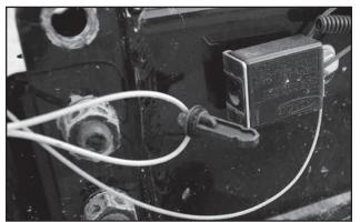
Fig 47 - Break-Away Switch Pin
