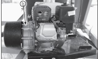
Fig 5 - Centrifugal Clutch
