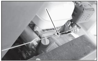
Fig 51 - Centrifugal Clutch
