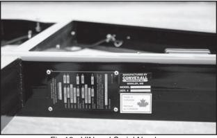
Fig 16 - VIN and Serial Number
