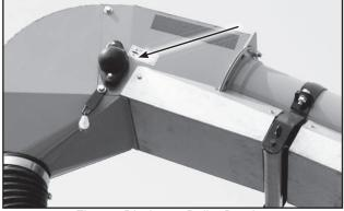
Fig 41 - Discharge Roller Bearing
