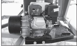
Fig 31 - Engine with Centrifugal Clutch
