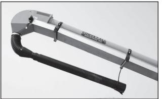
Fig 13 - Discharge Spout with Extension
