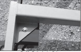
Fig 22 - Trailer Anchor Bolts
