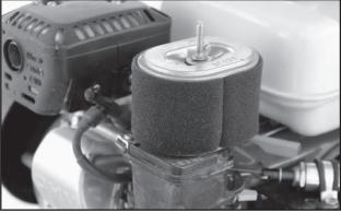
Fig 66 - Air Filter with Cover Removed
