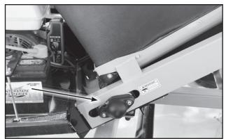
Fig 40 - Hopper Roller Bearing
