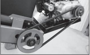
Fig 60 - Drive Belt, Guard Removed
