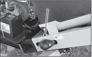
Fig 52 - Roller Bearing Housing, with Guard
