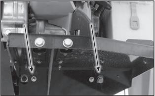
Fig 55 - Tension Bolts, Below Engine
