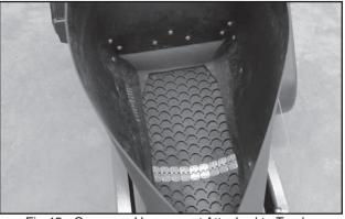
Fig 45 - Conveyor Hopper, not Attached to Tender
