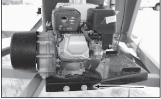
Fig 61 - Engine Mount Positioning Bolts
