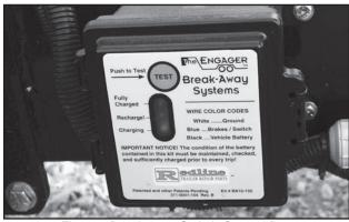
Fig 18 - Breakaway Switch Control Box
