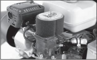
Fig 50 - Air Filter, Cover Removed
