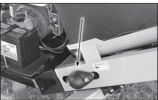
Fig 65 - Roller Bearing Housing, with Guard
