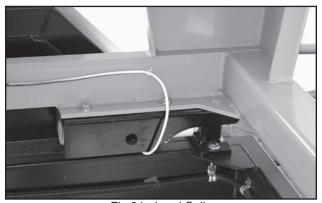
Fig 24 - Load Cells
