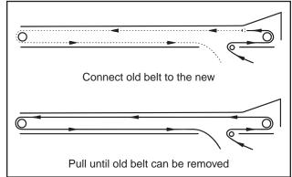
Fig 71 - Threading the Belt
