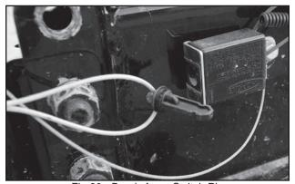
Fig 60 - Break-Away Switch Pin
