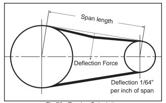
Fig 75 - Tension Calculation
