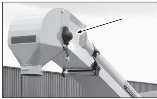
Fig 54 - Discharge Roller Bearing
