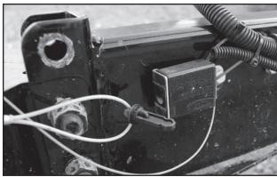
Fig 33 - Break-Away Switch with Pin Removed
