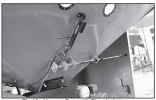
Fig 19 - Hopper Gate with Electric Actuator
