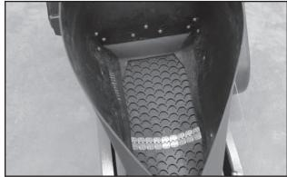
Fig 58 - Conveyor Hopper, Not Attached to Tender
