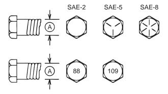
Torque figures indicated above are valid for non-greased or non-oiled threads and heads unless otherwise specified. Therefore, do not grease or oil bolts or capscrews unless otherwise specified in this manual. When using locking elements, increase torque values by 5%.
