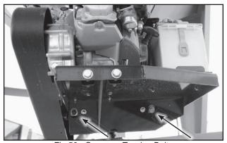
Fig 56 - Conveyor Tension Bolts
