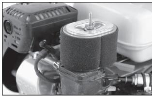
Fig 79 - Air Filter with Cover Removed
