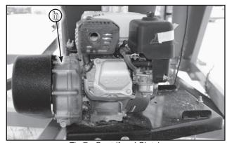
Fig 7 - Centrifugal Clutch
