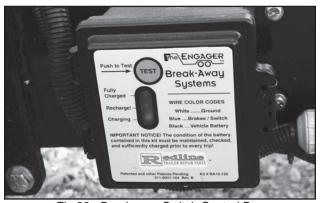
Fig 32 - Breakaway Switch Control Box
