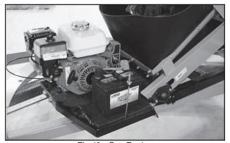
Fig 43 - Gas Engine
