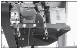
Fig 66 - Tension Bolts, Below Engine
