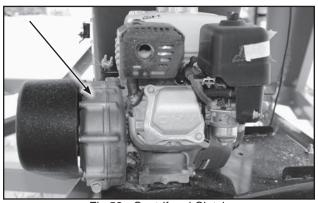
Fig 52 - Centrifugal Clutch
