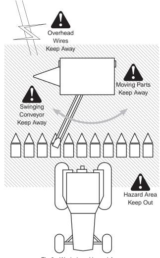
Fig 2 - Workplace Hazard Area
