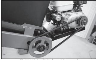
Fig 57 - Drive Belt, Guard Removed
