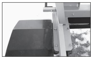
Fig 36 - Trailer Anchor Bolts
