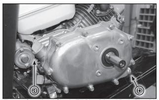
Fig 80 - Centrifugal Clutch, Fill Plug (a) and Drain Plug (b)
