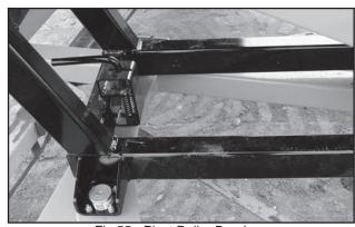
Fig 55 - Pivot Roller Bearings
