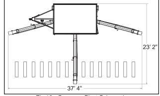
Fig 16 - Conveyor Pivot Schematic
