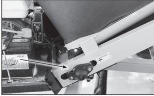
Fig 53 - Hopper Roller Bearing
