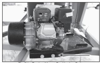
Fig 74 - Engine Mount Positioning Bolts
