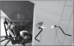
Fig 18 - Hopper Gate with Manual Levers
