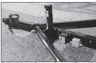
Fig 31 - Hitch, Jack, Breakaway System and Electrical Box
