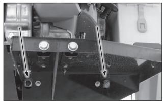
Fig 68 - Tension Bolts, Below Engine
