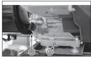
Fig 78 - Engine Oil, Fill Plug (a) and Drain Plug (b)
