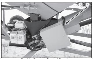
Fig 12 - Remote Control Receiver
