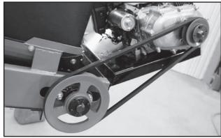
Fig 73 - Drive Belt, Guard Removed
