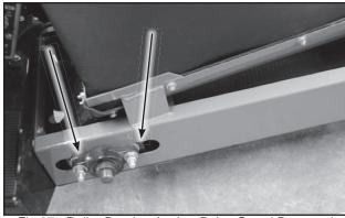
Fig 67 - Roller Bearing Anchor Bolts, Guard Removed
