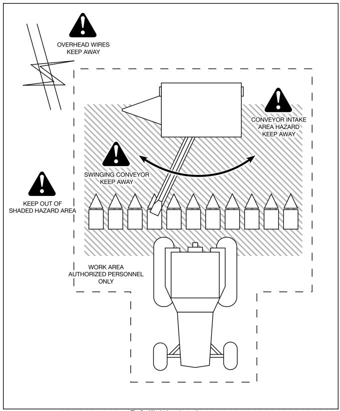
Fig 2 - Workplace hazard area
