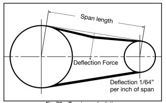
Fig 73 - Tension calculation
