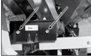
Fig 51 - Pivot roller bearings
