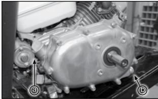
Fig 78 - Centrifugal Clutch - Fill Plug (a) and Drain Plug (b)
