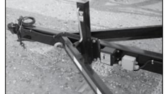
Fig 25 - Hitch, jack, breakaway system and electrical box
