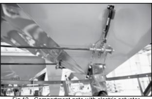
Fig 12 - Compartment gate with electric actuator
