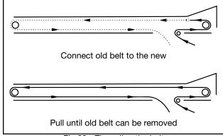
Fig 68 - Threading the belt
