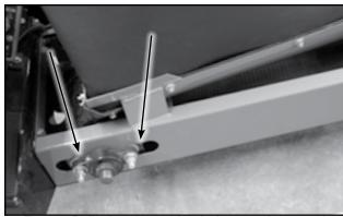
Fig 64 - Roller bearing anchor bolts, guard removed
