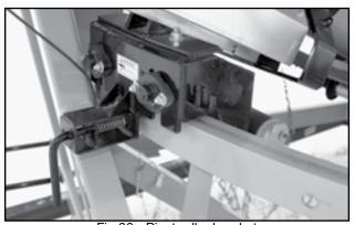
Fig 36 - Pivot roller bracket
