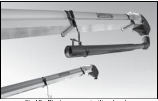
Fig 19 - Discharge spout with extension
