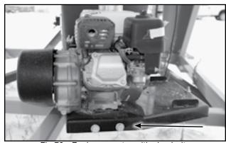
Fig 72 - Engine mount positioning bolts
