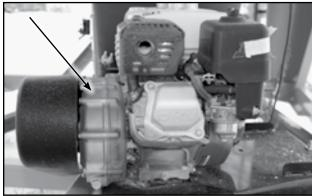
Fig 48 - Centrifugal clutch
