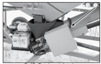
Fig 17 - Remote control receiver
