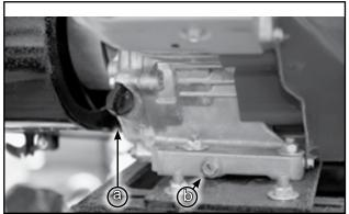
Fig 76 - Engine Oil - Fill Plug (a) and Drain Plug (b)
