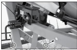
Fig 10 - Roller bracket pin (a), hole (b)
