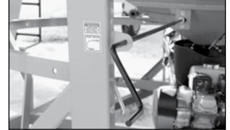
Fig 13 - Compartment gate with manual lever
