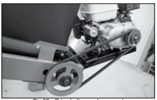
Fig 52 - Drive belt, guard removed
