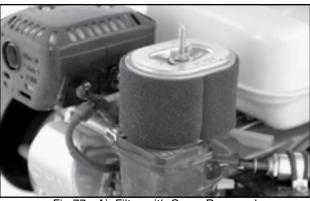
Fig 77 - Air Filter with Cover Removed
