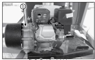
Fig 7 - Centrifugal clutch
