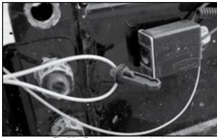
Fig 56 - Break-away switch pin
