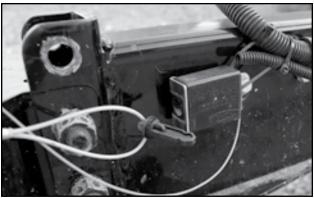
Fig 27 - Break-away switch with pin removed
