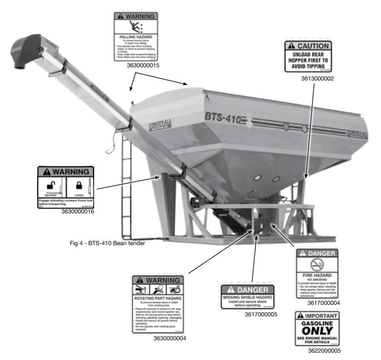
REMEMBER - If safety decals have been damaged, removed, become illegible, or parts were replaced without signage, new decals must be applied. Decals are available from your authorized dealer.
