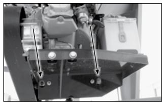
Fig 63 - Tension bolts, below engine
