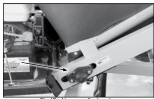
Fig 49 - Hopper roller bearing
