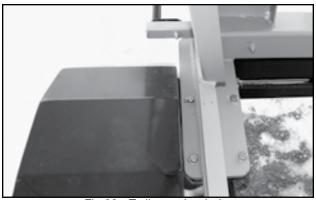
Fig 30 - Trailer anchor bolts
