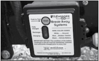
Fig 26 - Breakaway switch control box
