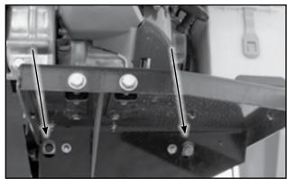
Fig 65 - Tension bolts, below engine
