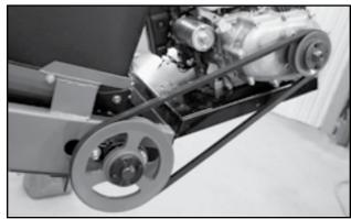
Fig 71 - Drive belt, guard removed
