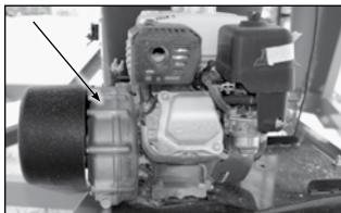
Fig 60 - Centrifugal clutch
