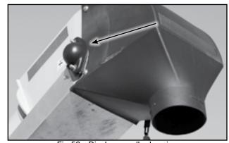
Fig 50 - Discharge roller bearing
