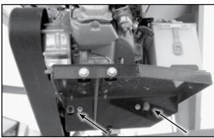
Fig 53 - Conveyor tension bolts
