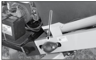
Fig 62 - Roller bearing housing, with guard
