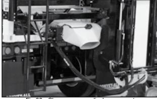
Fig 20 - Slave conveyor discharge spout
