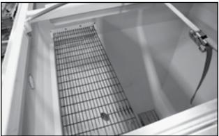
Fig 16 - Hopper catwalk
