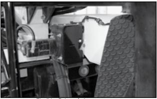
Fig 51 - Drive of slave conveyor
