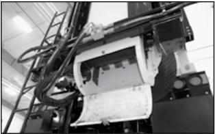
Fig 66 - Access door on folding conveyor
