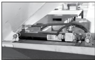
Fig 38 - Hopper discharge gate cylinder
