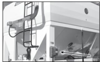
Fig 12 - Roll-top tarp controls
