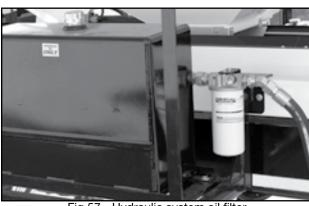
Fig 57 - Hydraulic system oil filter
