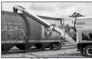
Fig 40 - Filling railcar
