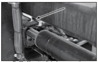
Fig 28 - Alternate cylinder frame connection
