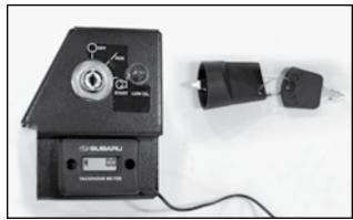
Fig 5 - Gas engine ignition switch
