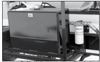
Fig 59 - Hydraulic reservoir and filter
