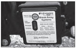
Fig 16 - Breakaway Switch Control Box
