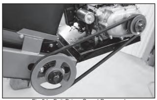
Fig 54 - Belt Drive, Guard Removed
