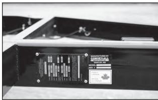
Fig 14 - VIN and Serial Number
