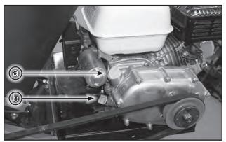
Fig 35 - Centrifugal Clutch Oil (a), Engine Oil (b)
