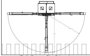
Fig 8 - Conveyor Pivot Schematic
