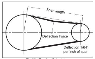
Fig 55 - Tension Calculation
