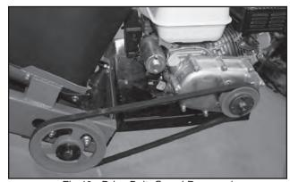
Fig 40 - Drive Belt, Guard Removed
