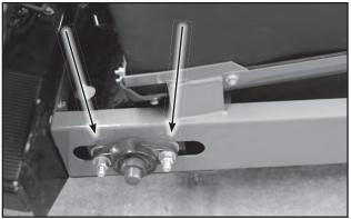
Fig 46 - Roller Bearing Anchor Bolts, Guard Removed
