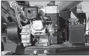
Fig 6 - Centrifugal Clutch
