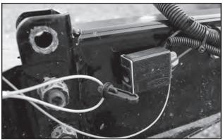
Fig 17 - Break-Away Switch with Pin Removed
