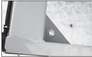
Fig 20 - Trailer Anchor Bolts
