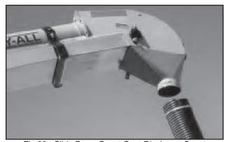
Fig 22 - Slide Down Spout Over Discharge Spout
