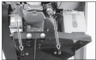
Fig 47 - Tension Bolts, Drive Roller
