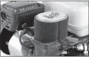
Fig 58 - Air Filter with Cover Removed
