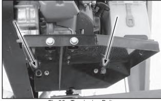
Fig 38 - Tensioning Bolts
