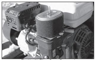
Fig 41 - Air Filter, Cover Removed
