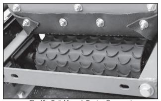
Fig 48 - Belt Aligned, Engine Removed
