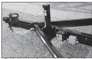
Fig 15 - Hitch, Jack, Breakaway System, Electrical Box
