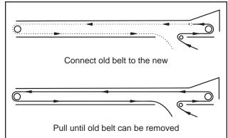
Fig 51 - Threading the Belt
