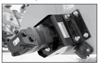
Fig 8 - Hydraulic motor, hoses not attached
