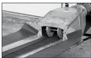
Fig 12 - Railcar hopper with hold-down wheels
