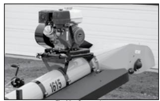
Fig 23 - Gas engine
