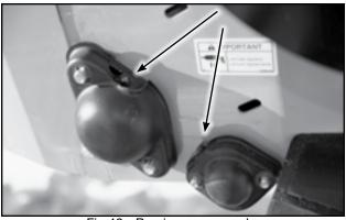
Fig 40 - Bearing grease zerks
