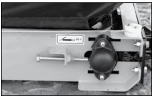
Fig 48 - Roller bearing mounts and anchor bolts
