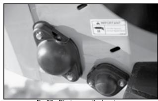
Fig 36 - Discharge roller bearings
