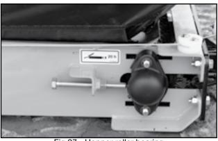
Fig 37 - Hopper roller bearing
