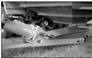
Fig 19 - Hopper sides raised
