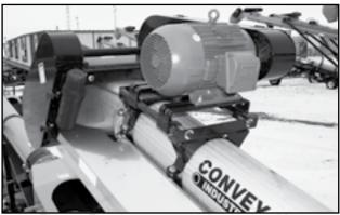
Fig 57 - Electric motor, speed reduction drive
