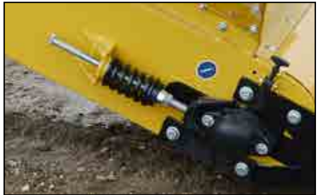
Fig 40 - Adjustment bolt and tension spring
