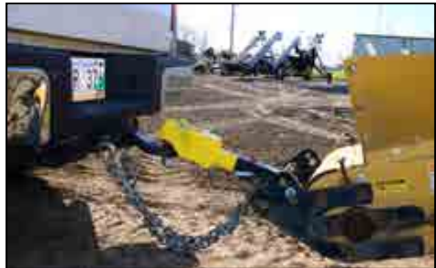
Fig 29 - Ball hitch with safety chains
