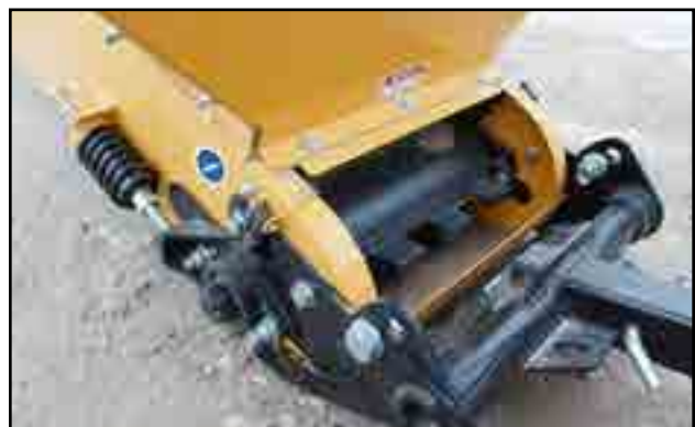
Fig 13 - Adjustable hitch. Belt guard is shown removed
