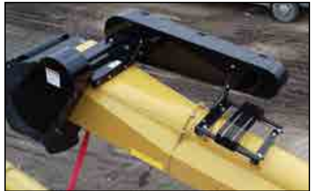
Fig 7 - Speed reducer with counter shaft
