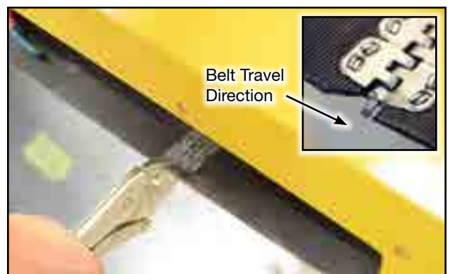
Fig 46 - Crimp lacing and taper belt corner
