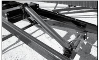
Fig 75 - Conveyor tube lift cylinder
