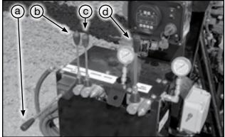
Fig 13 - Hydraulic levers
