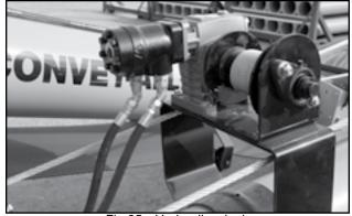
Fig 35 - Hydraulic winch
