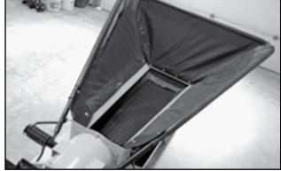
Fig 19 - Standard collapsible hopper
