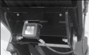
Fig 25 - Discharge working light
