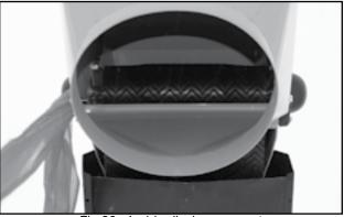
Fig 86 - Inside discharge spout
