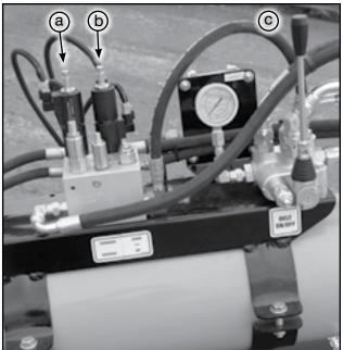
Fig 44 - Remote control valve table
