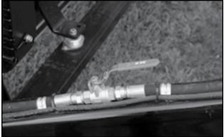
Fig 52 - Hydraulic ball valve to tube lift cylinder
