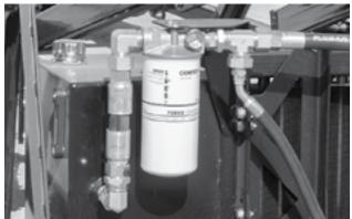
Fig 96 - Hydraulic oil filter
