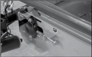
Fig 81 - Swing-out hopper roller bearing
