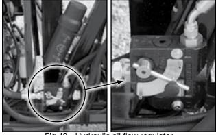
Fig 43 - Hydraulic oil flow regulator
