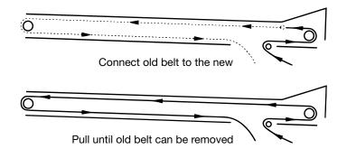
Fig 88 - Thread belt through conveyor
