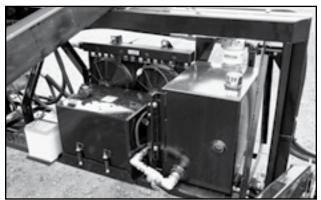
Fig 11 - Fuel tank and hydraulic reservoir
