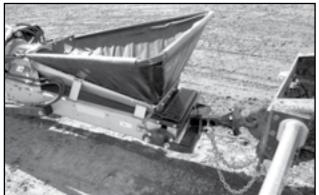
Fig 48 - Safety chain secured
