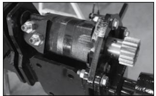
Fig 104 - Pinion gear
