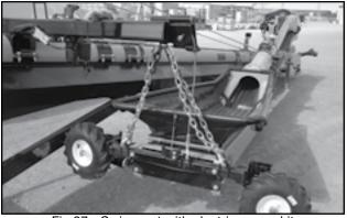
Fig 37 - Swing-out with electric mover kit
