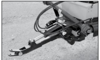
Fig 26 - 2200 series hydraulic hitch
