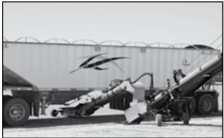
Fig 54 - Trailer unloading into swing-out conveyor
