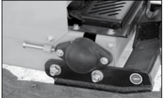
Fig 82 - Adjustment bolt on side of hopper
