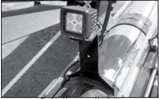
Fig 24 - Hopper working light
