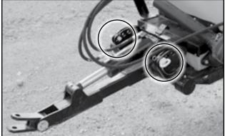
Fig 51 - Transport pins on hydraulic hitch
