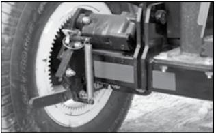
Fig 67 - Sprockets on drive wheel
