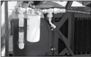
Fig 72 - Hydraulic oil filter
