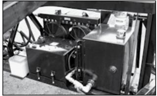
Fig 61 - Hydraulic oil reservoir and fuel tank
