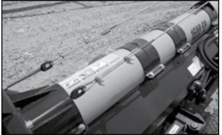
Fig 76 - Eyebolts and cable bridging
