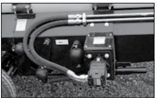
Fig 18 - Drive box with hydraulic motor
