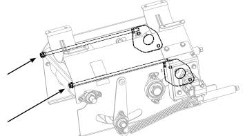
Fig 85 - Adjustment bolts and brackets inside drive box
