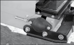
Fig 63 - Hopper roller bearings
