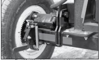
Fig 105 - Wheel ring gear and drive motor
