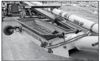
Fig 71 - Swing-out conveyor
