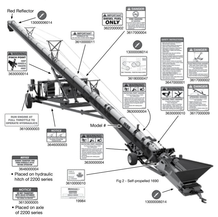
REMEMBER - If safety decals have been damaged, removed, become illegible, or parts were replaced without signage, new ones must be applied. New decals are available from your authorized dealer.
