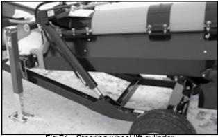
Fig 74 - Steering wheel lift cylinder
