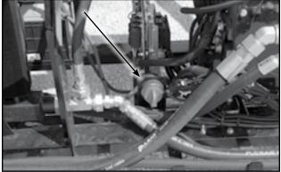
Fig 9 - Power shut-off switch
