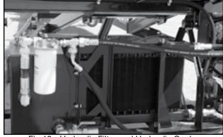
Fig 12 - Hydraulic Filter and Hydraulic Cooler
