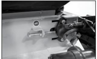
Fig 87 - Adjustment bolts on the swing-out
