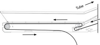
Fig 91 - Threading belt around hopper
