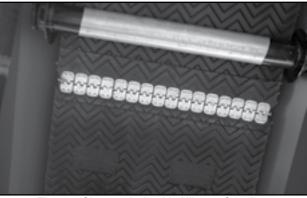
Fig 21 - Chevron belt with Alligator® lacing
