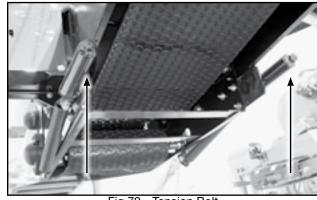
Fig 79 - Tension Bolt
