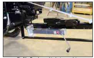
Fig 51 - Drawbar and jack storage plate
