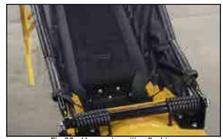
Fig 36 - Hopper transition flashing
