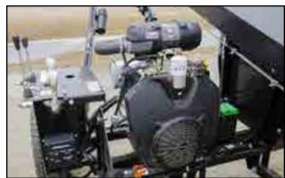
Fig 6 - Gas engine
