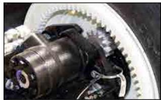
Fig 115 - Ring gear and pinion gear
