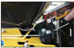
Fig 111 - Silicone gap in front corners
