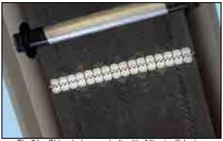
Fig 21 - Skived chevron belt with Alligator® lacing
