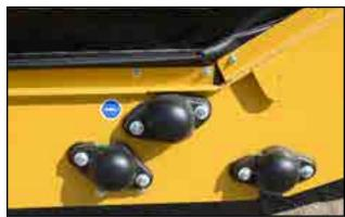
Fig 63 - Transition roller bearings
