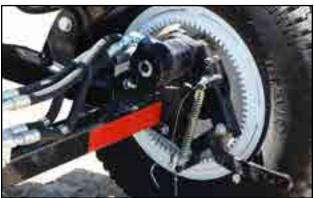
Fig 113 - Wheel ring gear and drive motor
