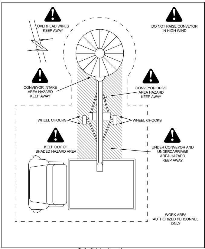
Fig 3 - Workplace Hazard Area
