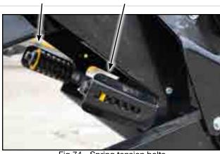
Fig 74 - Spring tension bolts
