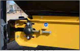
Fig 62 - Tail roller bearing
