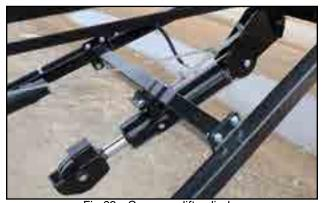
Fig 69 - Conveyor lift cylinder
