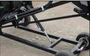
Fig 68 - Steering wheel lift cylinder
