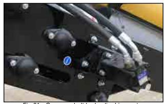
Fig 61 - Conveyor belt hydraulic drive motor
