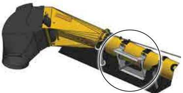
Fig 33 - Belt scraper after the discharge
