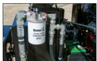
Fig 89 - Hydraulic Oil Filter
