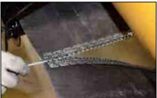
Fig 87 - Thread lacing cable
