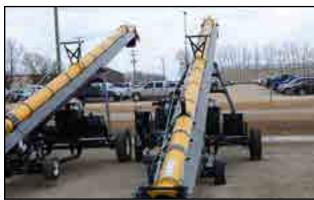
Fig 71 - Straight conveyor tube
