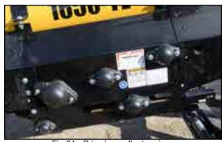
Fig 64 - Drive box roller bearings
