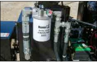
Fig 66 - Hydraulic filter
