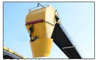
Fig 28 - Quad-swivel discharge spout and transport lights
