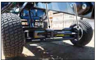
Fig 67 - Steering wheel axle bushings
