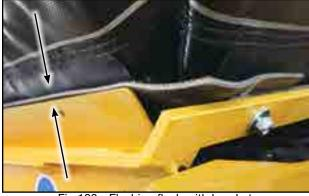
Fig 103 - Flashing flush with brackets
