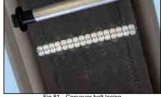
Fig 81 - Conveyor belt lacing
