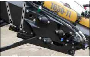
Fig 58 - Spring tension bolts, below drive box
