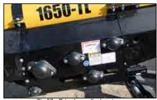
Fig 57 - Drive box roller bearings
