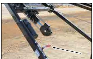
Fig 16 - Lift cylinder and ball valve
