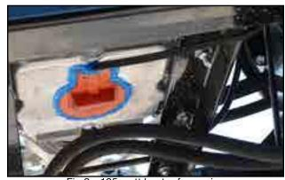
Fig 9 - 125 watt heater for engine
