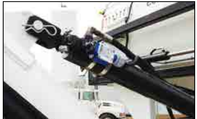
Fig 23 - Discharge raise limit switch (L4)
