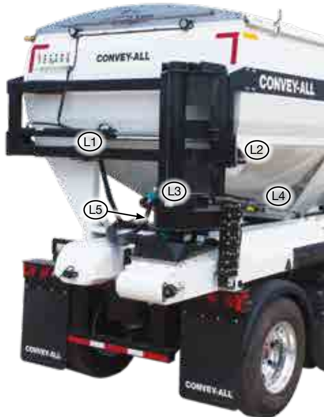
Fig 19 - Limit switches controlling rear conveyor movements
