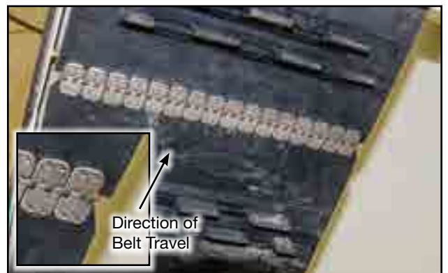
Fig 71 - Alligator lacing on rear conveyor paddle belt
