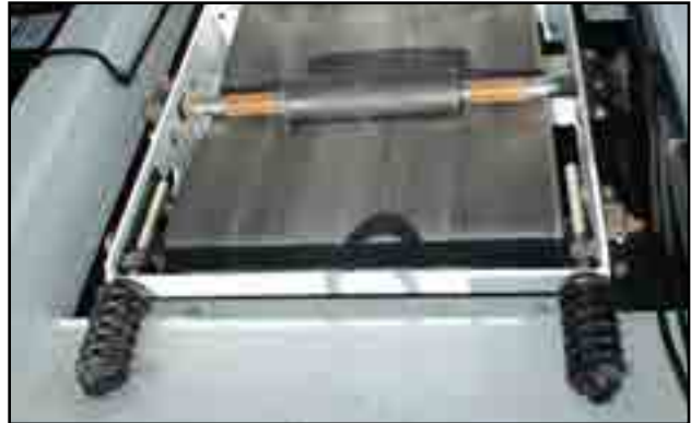
Fig 60 - Slave conveyor tension bolts, belt cover removed
