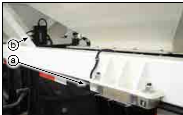
Fig 18 - (a) Load Cell, (b) weigh scale junction box
